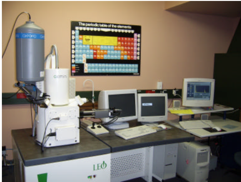
Figure 5: SEM system used for measurements at the CSIR-NML Pretoria.
