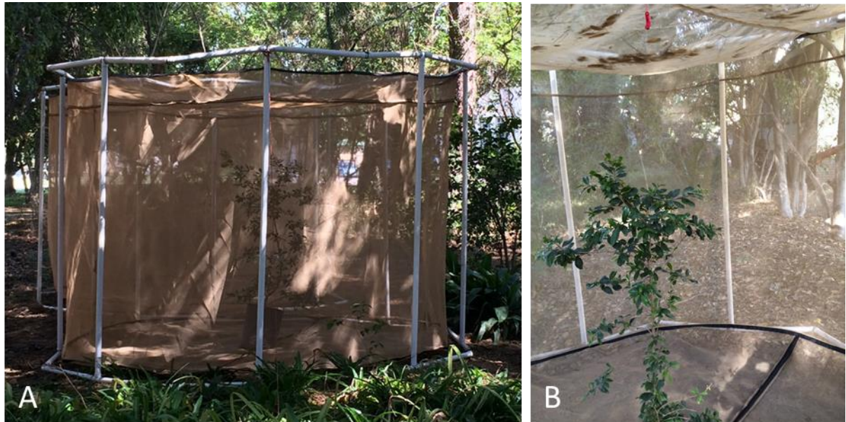
Fig. 6.1. The outside (A) and inside (B) of a cylindrical walk-in field cage, made of panels of polyester netting joined with black nylon strips, deployed in a small forest at the ARC-OVI, Pretoria, South Africa.
