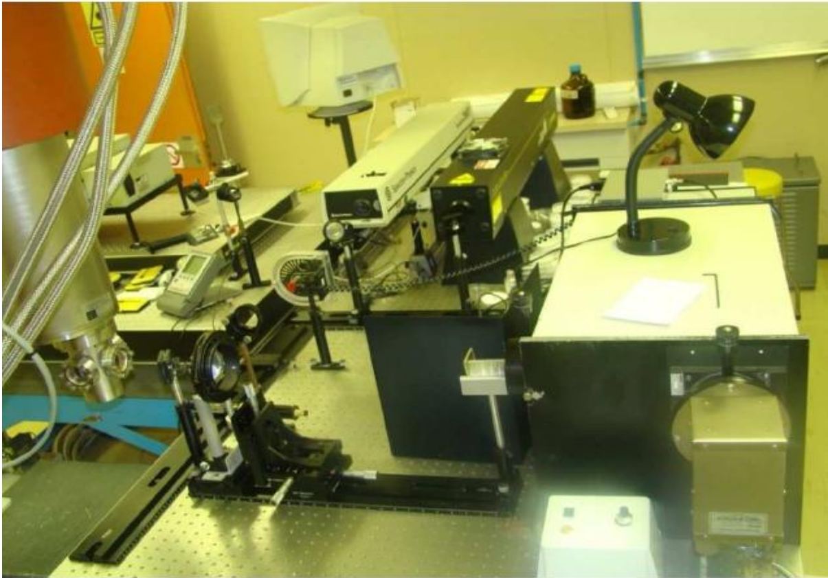
Figure 2.12: He-Cd laser (325 nm) photoluminescent system used to investigate the luminescent properties of the phosphors.
