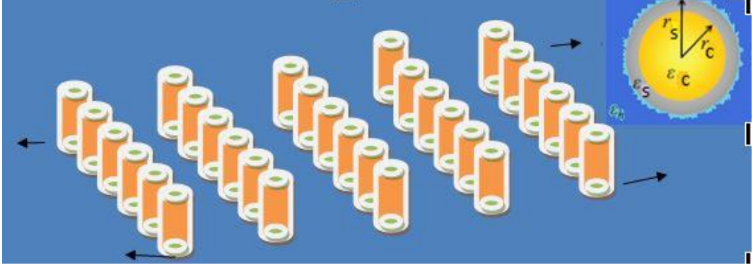
Figure 4.1: Structural model for cylindrical core-shell nanowire under consideration together with the relevant parameters.
