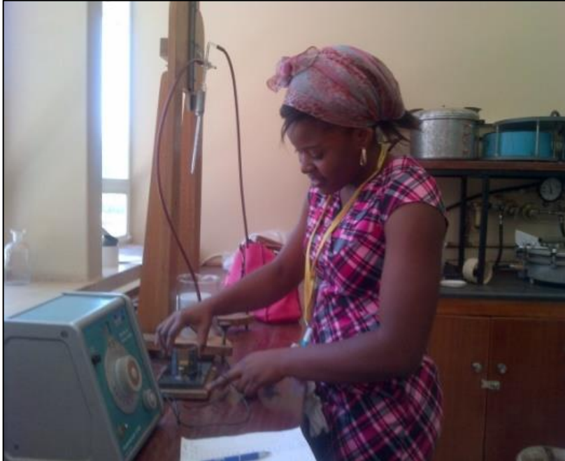
Figure 3.7 Using soil saturated pastes to determine soil resistivity.
