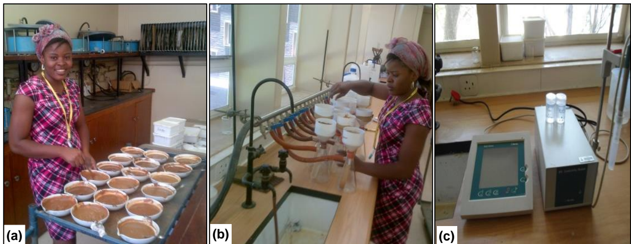
Figure 3.6 Laboratory preparations for EC_e measurement: (a) Saturating the soil samples, (b) setting up the Büchner funnels and flasks to the suction pipes, and (c) the Metrohm Module-856 conductivity meter for EC_e determination.
