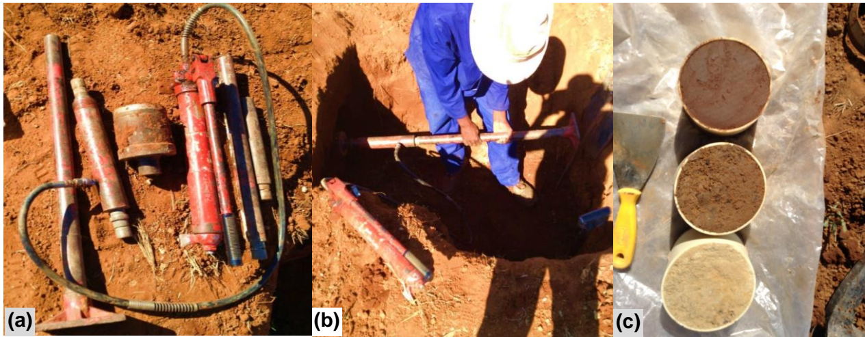
Figure 3.4 Field pictures showing the (a) Mechanical hydraulic-jack, (b) core sampling horizontally in the soil profile pit, and (c) the resulting soil core.
