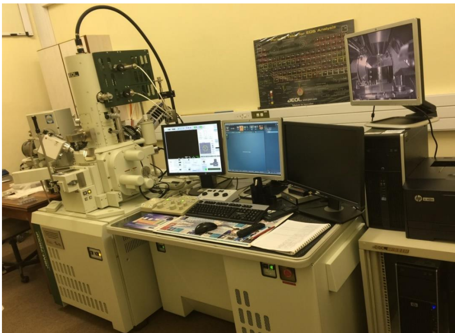
Figure 3.10: A typical SEM instrument, showing the electron column, sample chamber, EDS detector, electronics console, and visual display monitors.
