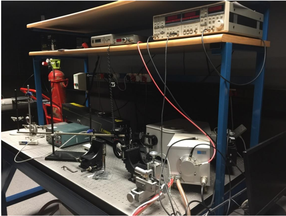
Figure 3.15 : A typical PL laser system with an excitation wavelength of 325 nm.
