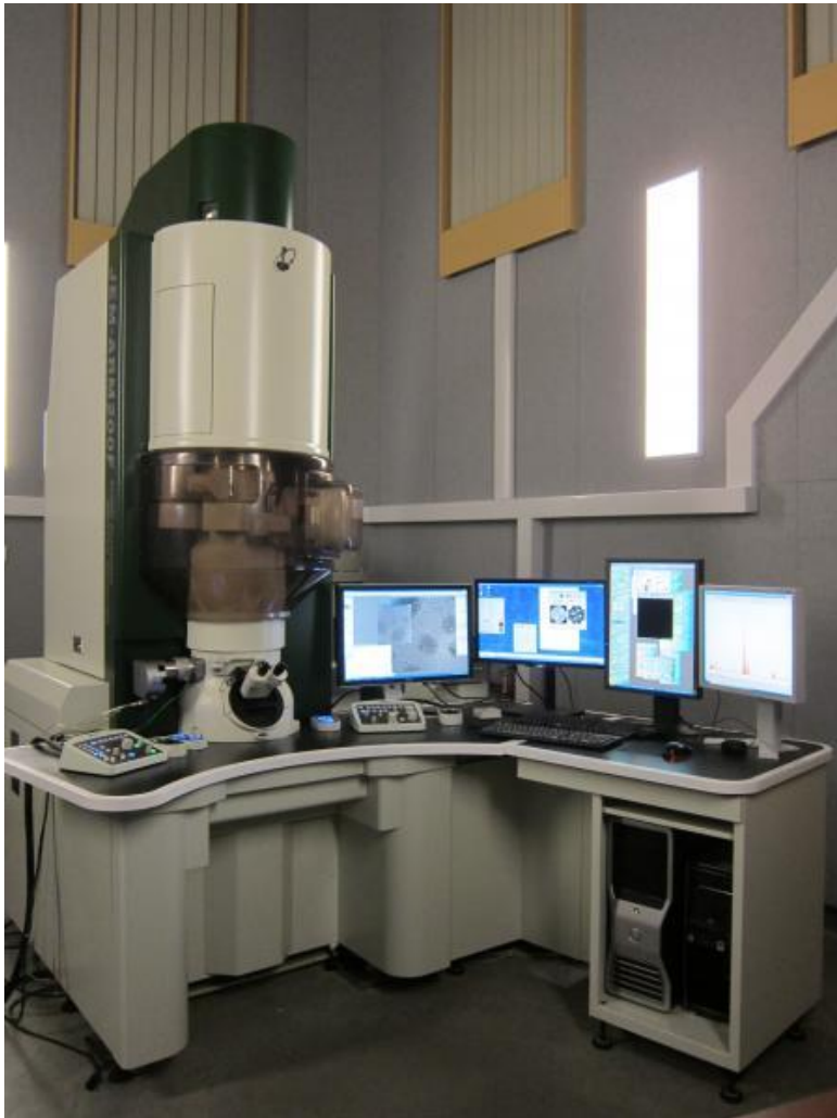
Figure 3.8: The JEOL JEM-ARM200F HR-TEM [24].
