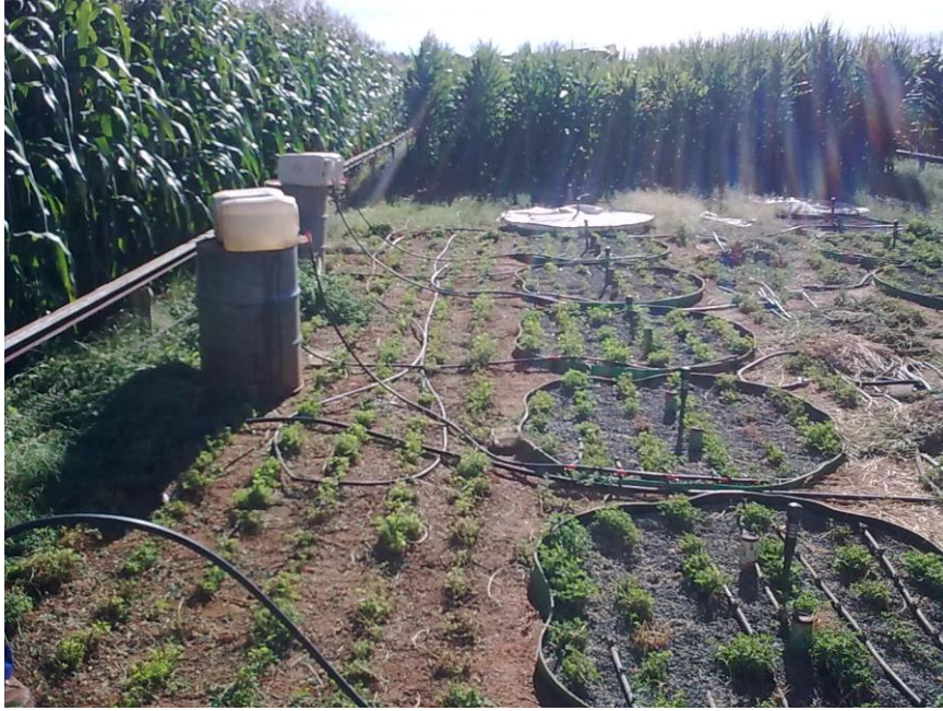
Figure 3.4 Surface driplines connected to the 20 L reservoirs for controlling the amount of irrigation of the different EC i treatments.
