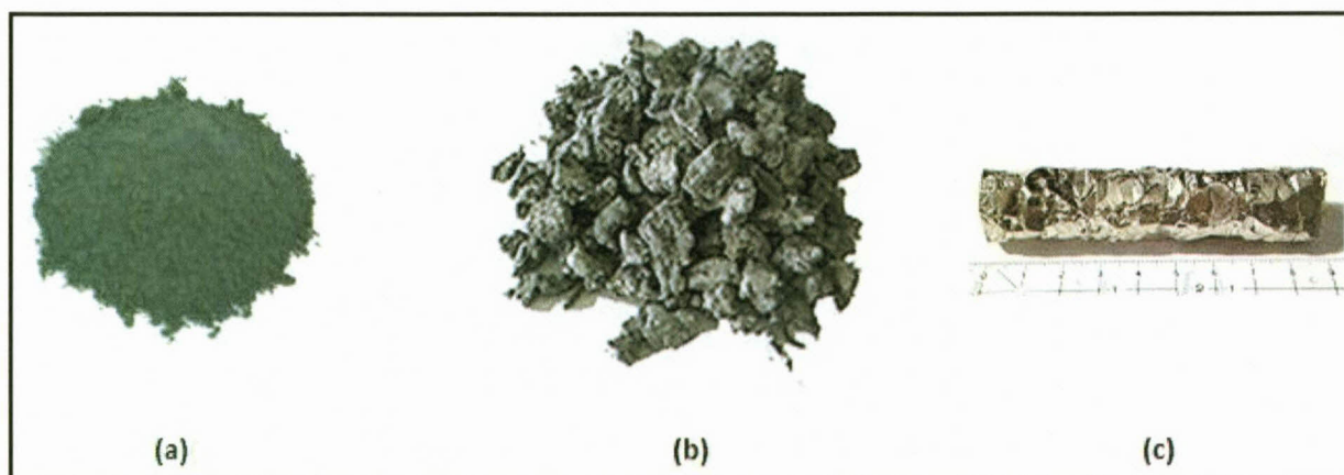
Figure 1.6: (a) Zirconium powder; (b) Zirconium sponge; (c) Zirconium crystal bar 2
