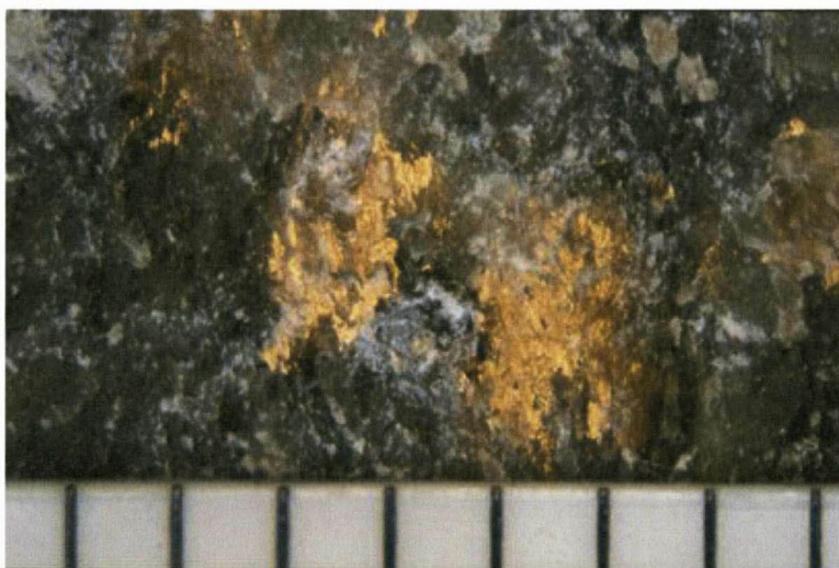
Figure 2-13 Gold ore sample from Gaika Reef (G24) located in the Midland Greenstone Belt (scale divisions = 2.5 mm).
