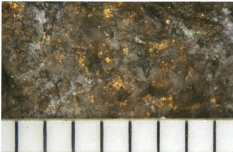
Figure 2-6 Gold ore sample from New Consort Mine (MGS10591) located in the Barberton Greenstone Belt (scale divisions = 2.5 mm).
