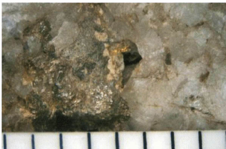
Figure 2-12 Gold ore sample from Knysna Mine (G111b) located in the Cape Supergroup (scale divisions = 2.5 mm).
