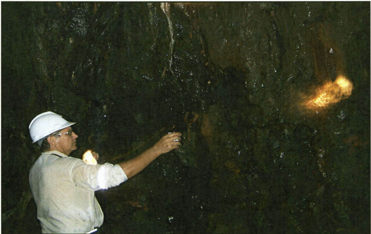
Figure 73: A sample being collected in the gold mine next to a fracture.
