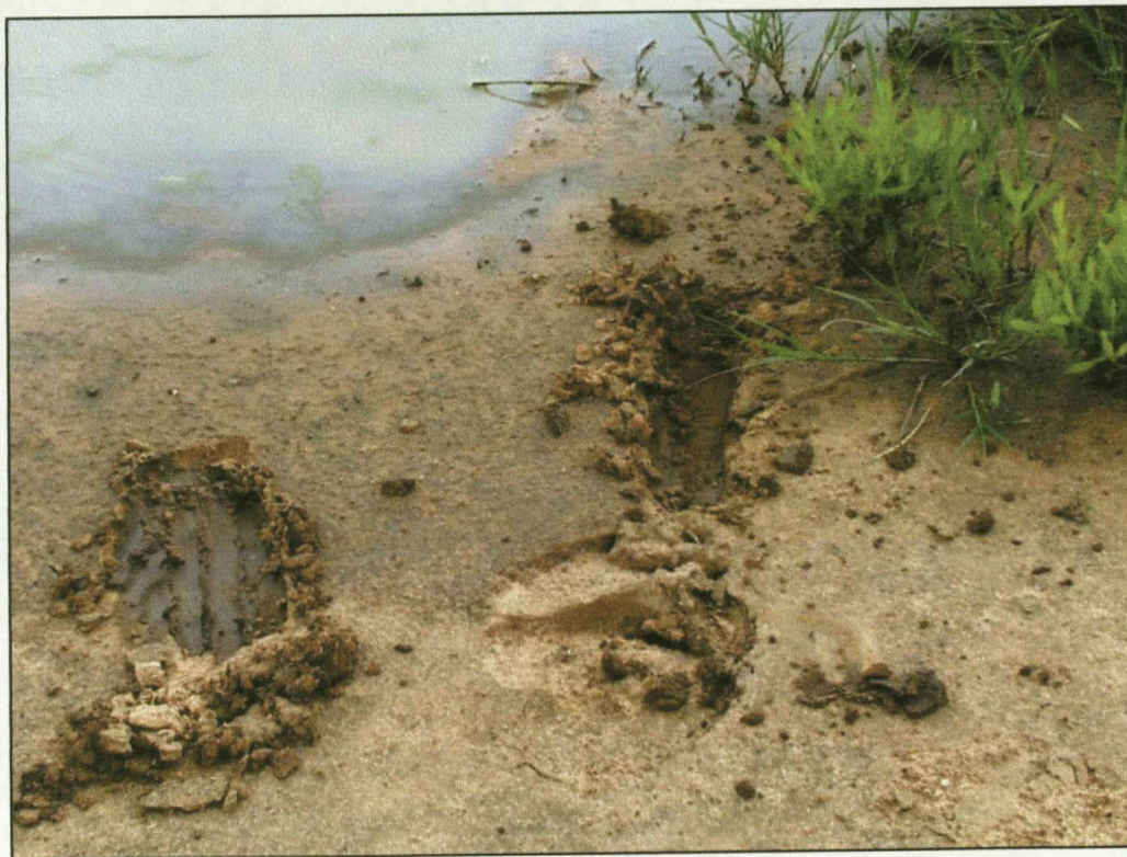
Plate 5.1 Soil near a small pan indicating a thin clay layer before going through into a coarse sand layer beneath the pan surface.
