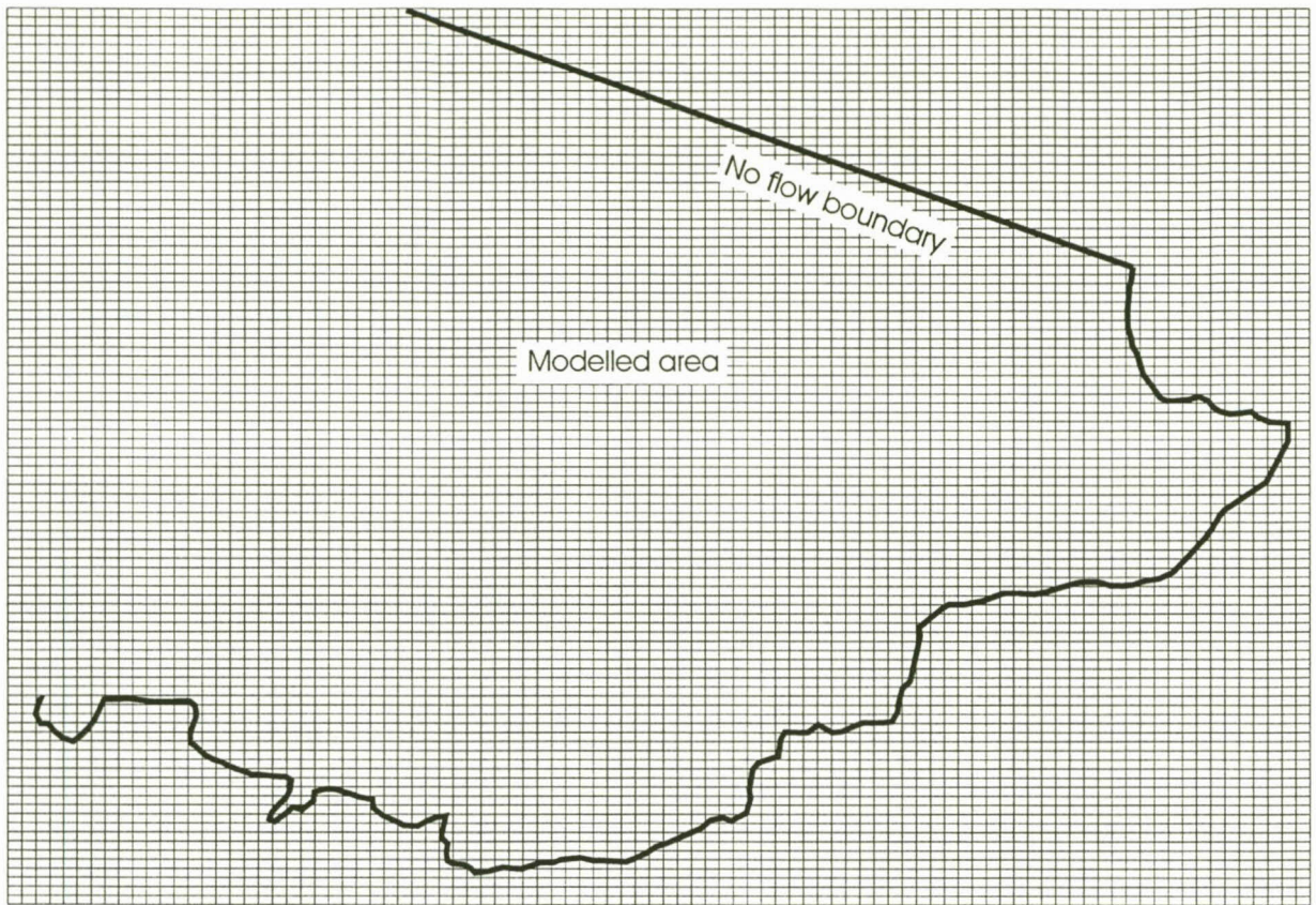
Figure 7.1 : Modelling network for the Struisbaai aquifer
