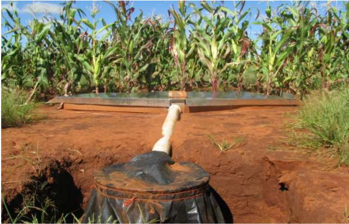
Figure 3. 11 Runoff strip with installed tipping bucket.
