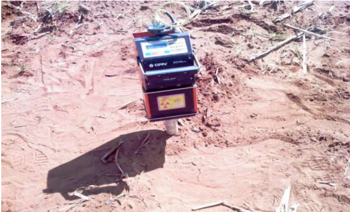
Figure 3. 10 Neutron water meter used to measure soil water content.
