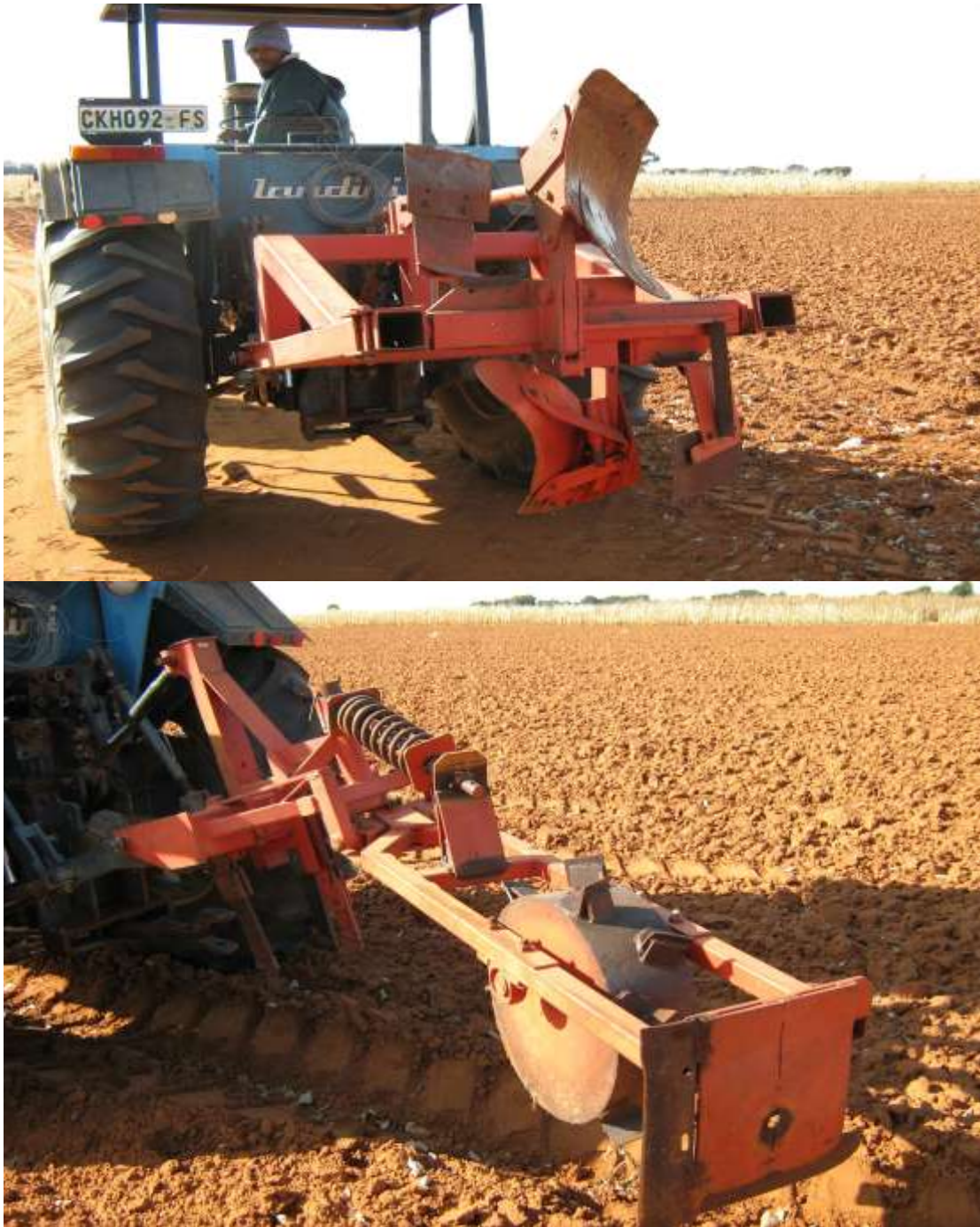
Figure 3. 6 Demonstration of ridge plough and the puddler plough all developed by Bramley Engineering in Bloemfontein (Bothma, 2009).
