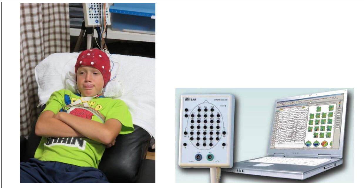
Figure 3: The EEG cap is connected to a MITSAR amplifier and an EEG recording computer (Image researcher's own with permission granted.)
