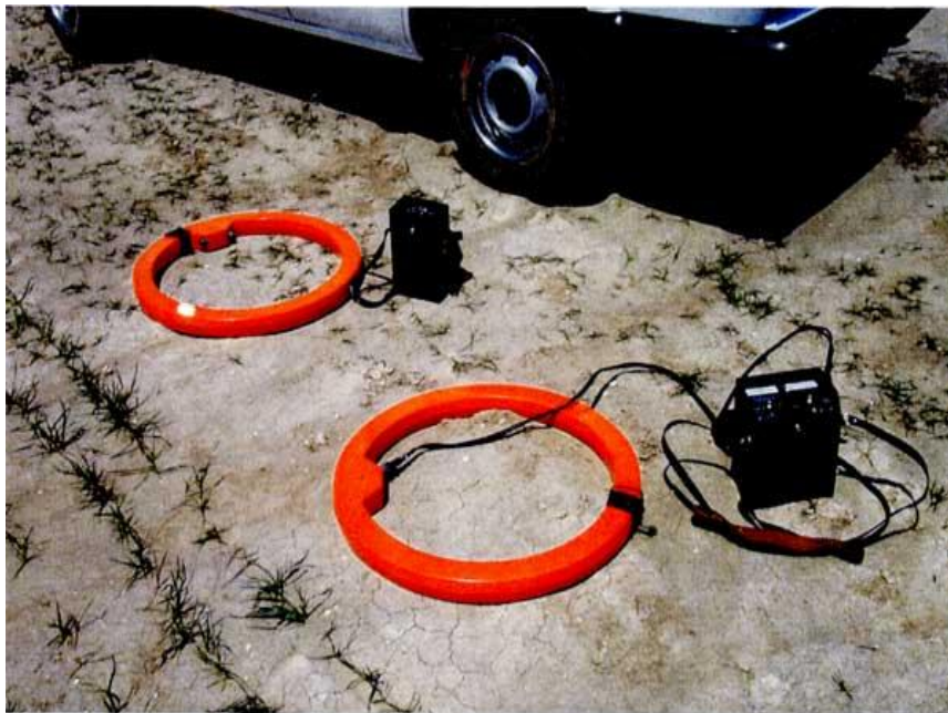
Figure 36: Terrain conductivity survey using the EM34-3 system in vertical dipole (horizontal coil) mode ( www.geonics.com )
