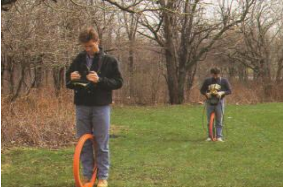
Figure 35: Terrain conductivity survey using the EM34-3 system in horizontal dipole (vertical coil) mode ( www.geonics.com )
