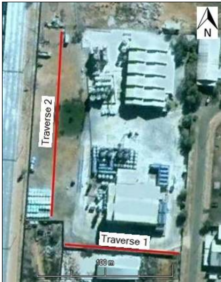
Figure 23: Two Dimensional Resistivity Traverses at the SNP Site.
