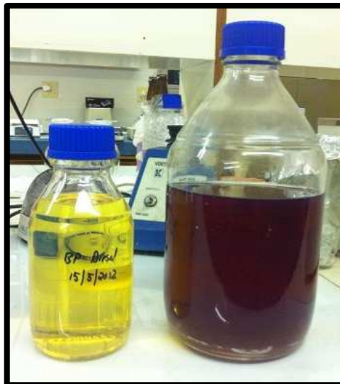
Figure 3.3: Microbial contaminated diesel sample obtained from Earthmoving Repair Services (sample on the right). Sample on the left is fresh commercial diesel.
