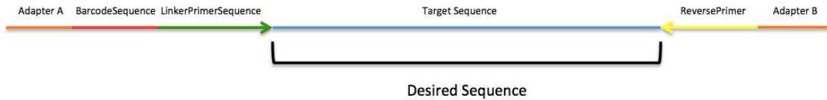
Figure 5.1: The primer construct and amplicon used in Illumina sequencing (taken from “Qiime,” 2015).
