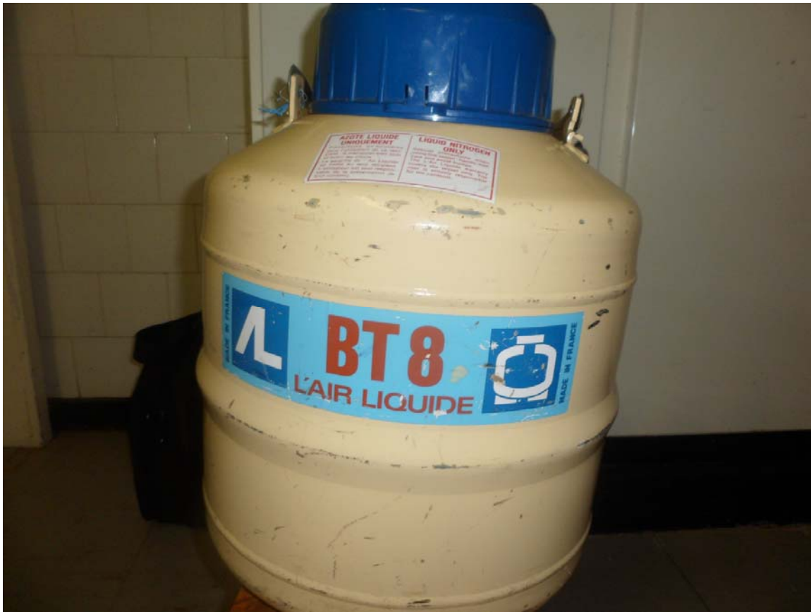
Plate 3.13 Liquid nitrogen tank used for the storage of semen after cryopreservation
