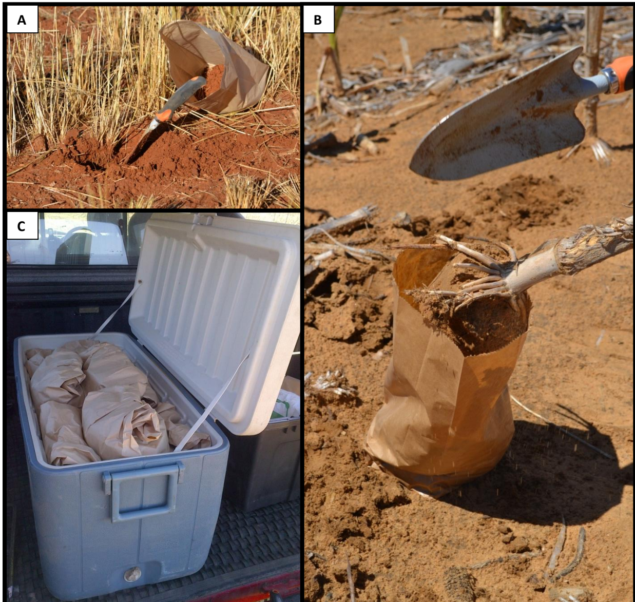
Fig. 2.1: Sampling procedure. A-B: sampling of soil from the porosphere of the plants by means of a trowel; C: transporting samples in a cooler box.
