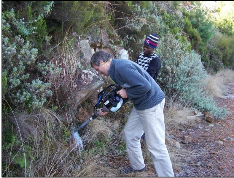
Figure 3.2: All cores for palaeomagnetic investigations were drilled in the field with a water-cooled portable rock drill. The sample sites were selected after in situ conditions for geographic orientation.
