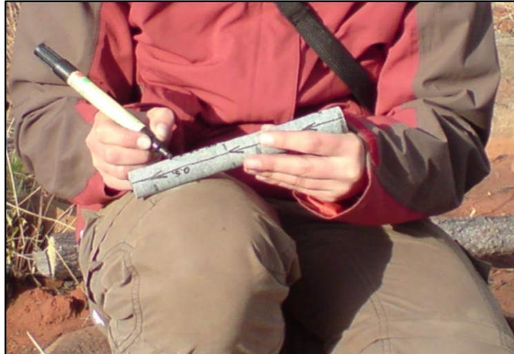
Figure 3.4: After orientation every core was labeled. The arrows marked the dipping direction.
