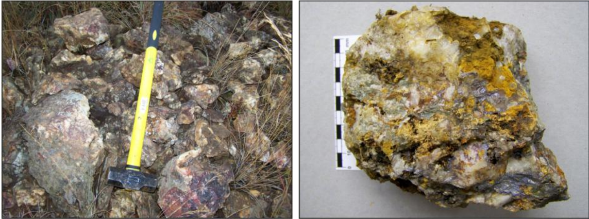
Figure 4.6: The Black Reef Quartzites occur in the footwall zone of the Uitkomst Complex on the farm Vaalkop and Uitkomst. Fritted quartzites (left) indicate the high thermal conditions due to the Intrusion. The hand specimens show boxwork structures caused by the weathering of the sulphides (right, VK_11-6_1/1). These boxes are covered by a coat of light brown iron oxides.
