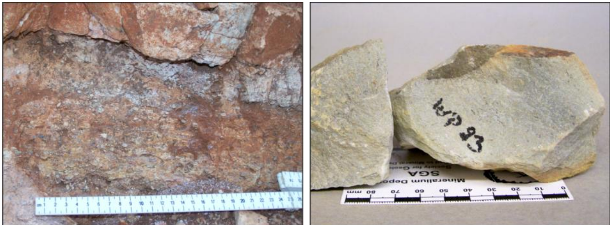
Figure 4.5: In contact with the overlying Malmani Dolomite the Black Reef Quartzites occurs as pebbly layers with a conglomerate like appearance (outcrop on the left is located on the farm Vaalkop). In hand specimen the fine grained quartzite has a creamy color with a slight greenish color cast (right).
