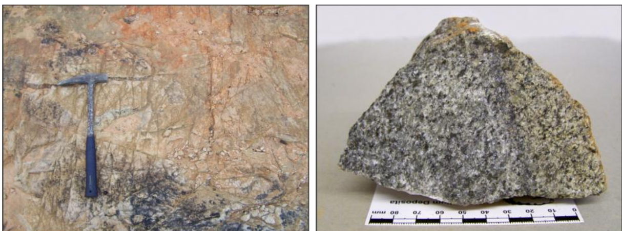
Figure 4.3: In outcrop the granite gneiss occurs as weathered orange blocky rocks, which are structured by many joints of different orientation (left picture, close up view from a big block of granite gneiss). In contrast the fresh hand specimen on the right shows a grey coloration interspersed with black biotite and hornblende. Compared to the mafic sills and dykes it is distinctively harder due to the high quartz content. The weakly foliation is defined by the planar alignment of biotite and hornblende components.
