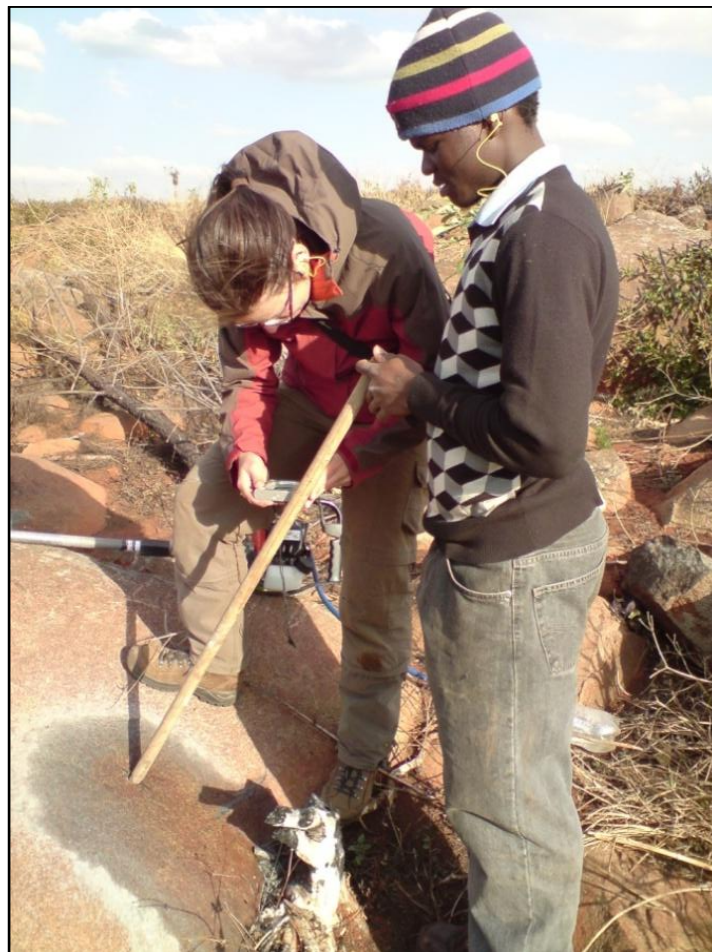
Figure 3.3: For orientation a geological compass combined with a wooden extension was used to exclude any measuring mistakes due to magnetization of the outcrop.
