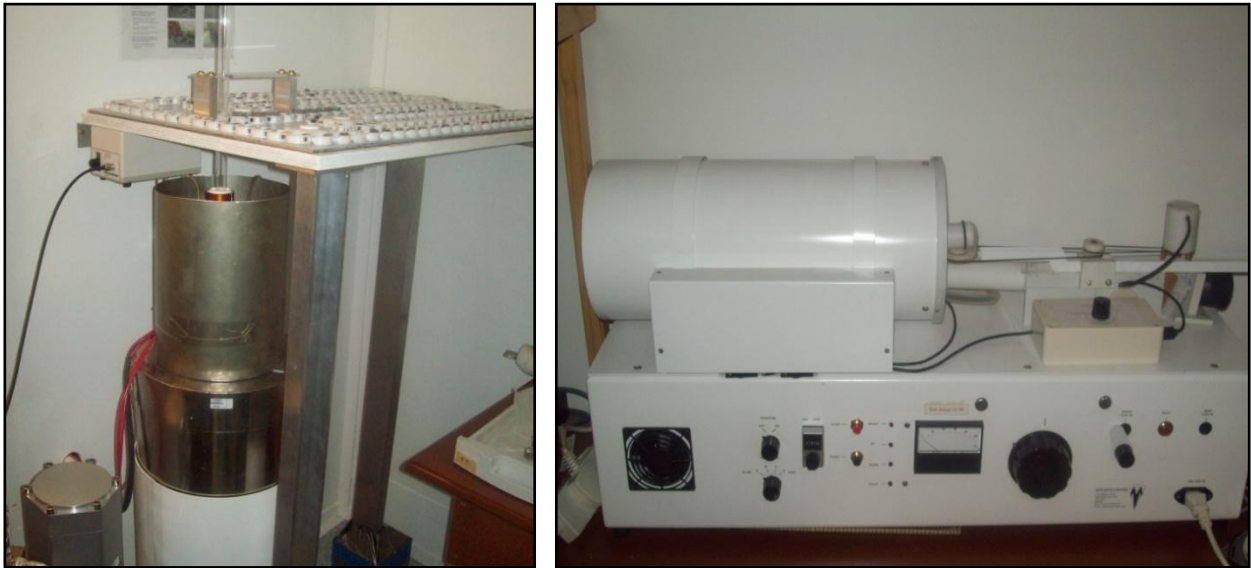
Figure 7.2: On the left the cryogenic magnetometer is shown, which measured the natural remanent magnetisation (NRM) of the samples. The following demagnetisation procedure was carried out on a Molspin two-axis tumbling Alternating-field (AF) - demagnetiser (right) (pictures by courtesy of Tumelo Mokgatle).
