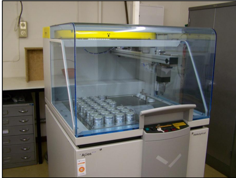
Figure 3.5: PANalytical WD-XRF Axios spectrometer
