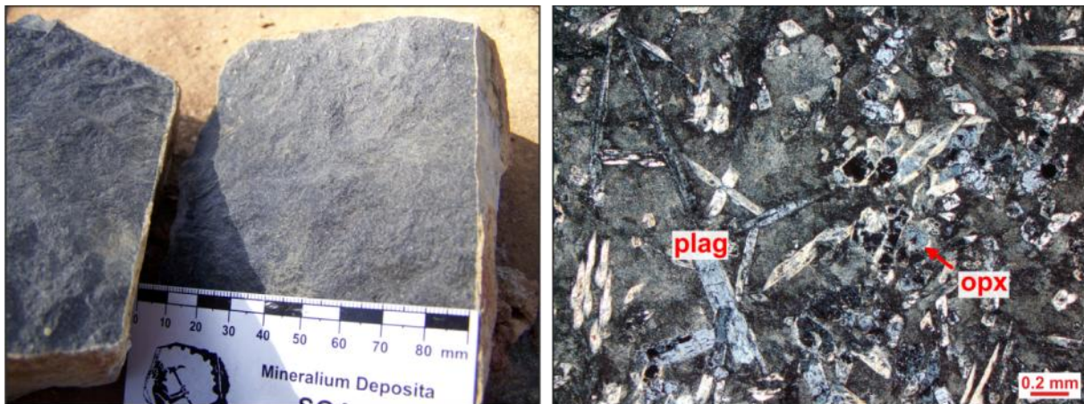
Figure 5.6: The hand specimen of the chilled margin of US-1 has a fine dark grey groundmass interspersed with fine light grey needles of feldspar. Notice the white film surrounding the sample on the left. Microscopically, the groundmass consists of variolitic plagioclase, quartz, alteration minerals and glass. Lath-shaped plagioclase and stubby prismatic orthopyroxene occur as phenocrysts within the groundmass (right picture, under XP view).
