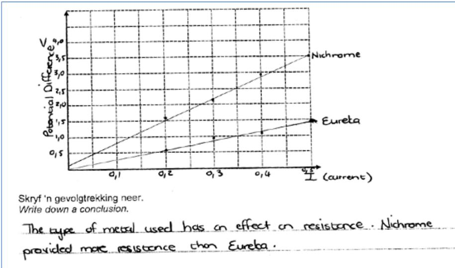
Figure 4: Experimental data are obtained to plot a graph at workstation 2
