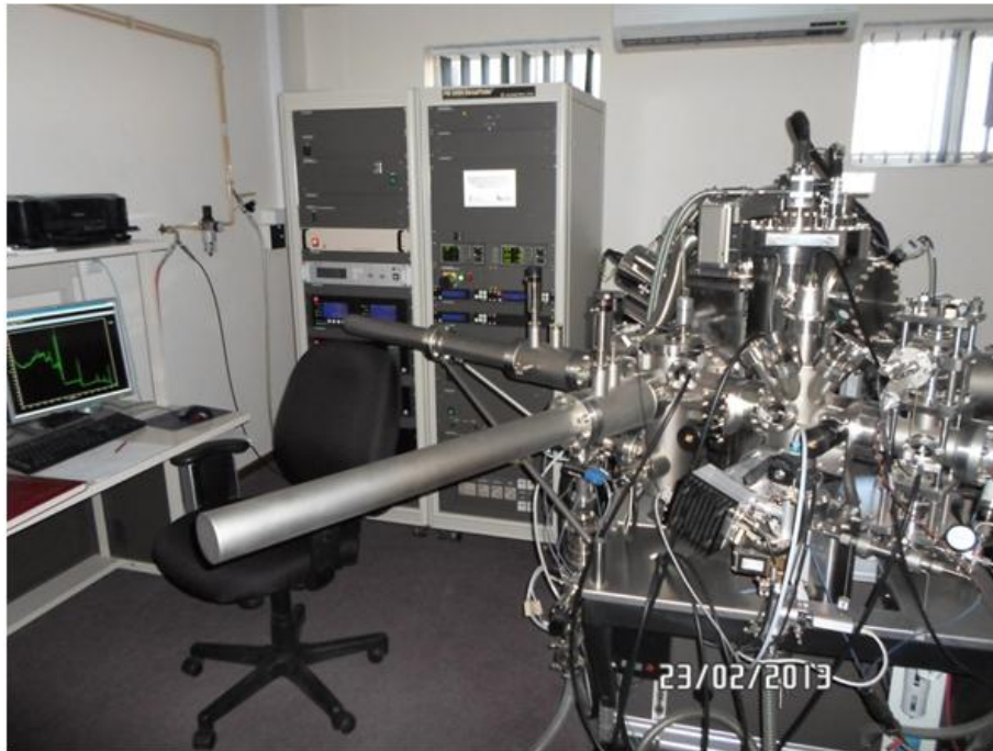
Figure 3.15: PHI 5000 Versaprobe XPS system at the Department of Physics, University of the Free State.
