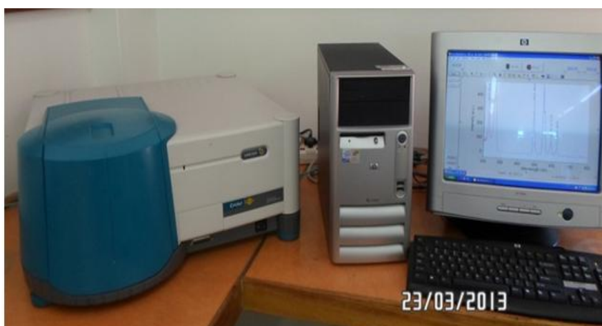
Figure 3.17: Cary Eclipse fluorescence spectrophotometer at the Department of Physics, University of the Free State.
