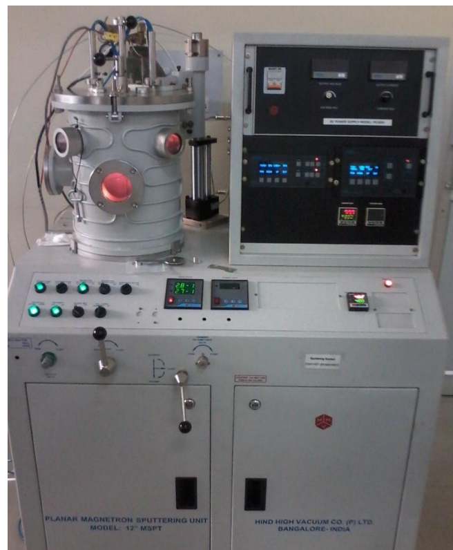
Figure 3.7: The system used for the RF magnetron technique at the Semiconductor Physics Lab, Department of Physics, Gurukula Kangri University, Haridwar, India.
