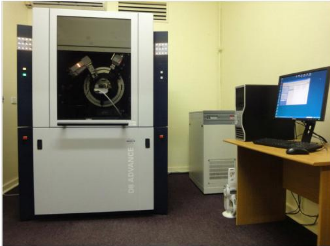
Figure 3.10: The Bruker D8 Advance x-ray diffractometer at the Department of Physics of the University of the Free State.
