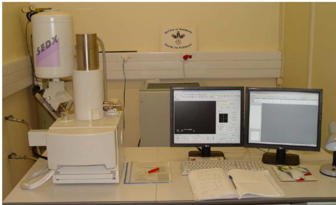
Figure 3.12: The Shimadzu Superscan SSX-550 SEM system at the centre for Microscopy, University of the Free State.
