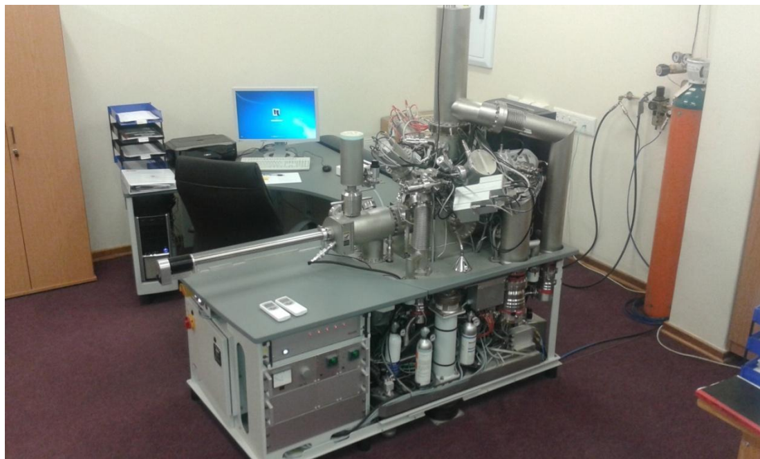
Figure 3.25: A photograph of the TOF-SIMS 5 at the Department of Physics, University of the Free State.
