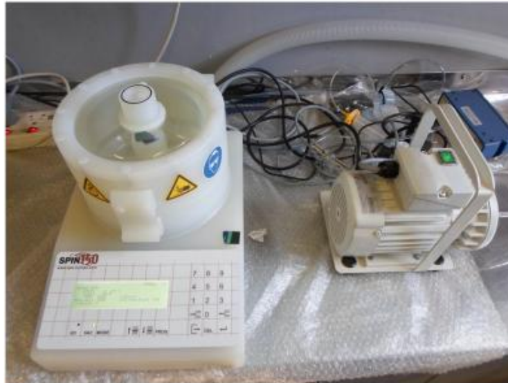
Figure 3.5: SPEN 150 spin coater from Semiconductor Production System at the Department of Physics of the University of the Free State.
