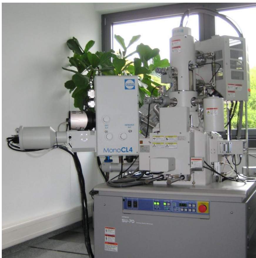
Figure 3.20: The MonoCL4 Elite installed on the Hitachi SU-70 SEM system.
