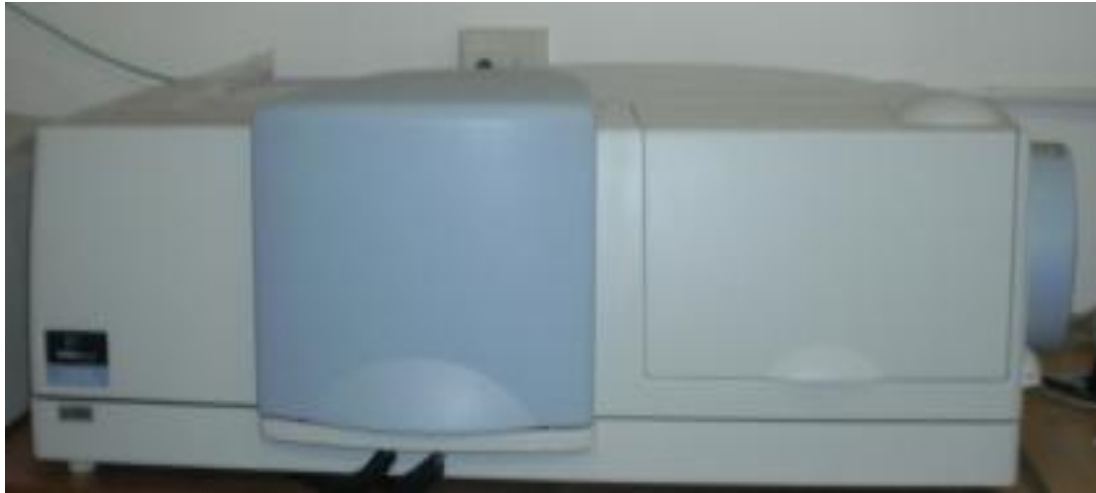
Figure 3.21: The Lambda 950 UV-Vis spectrophotometer at the Department of Physics of the University of the Free State.
