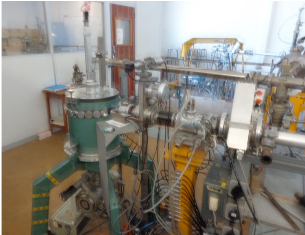
Figure 3.25: Photograph of the RBS system at the Ithemba Labs, Cape Town, South Africa.
