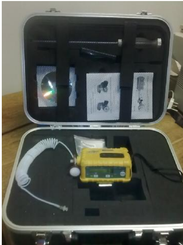
Figure 54: The Mini Rae Plus 3000 used in the soil vapour survey.
