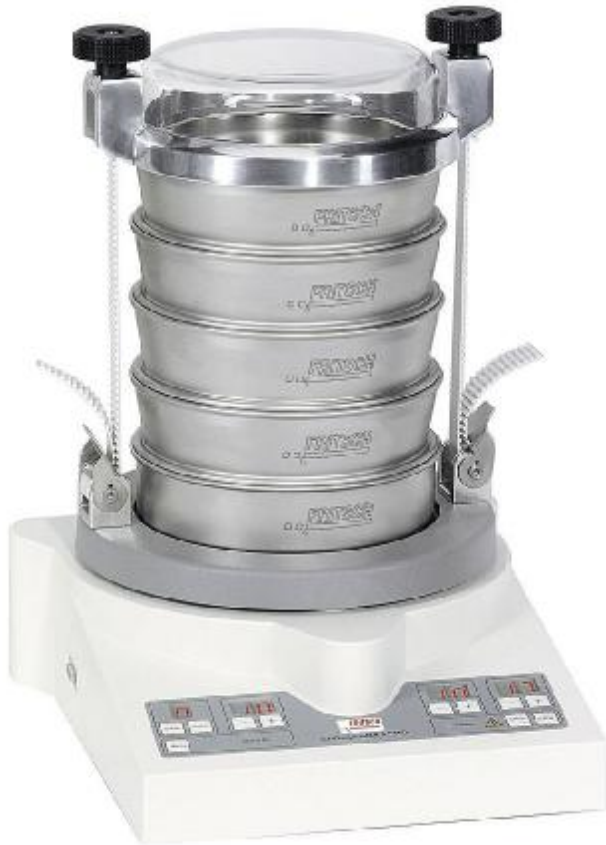
Figure 33: Sieve shaker used in the grain-size distribution analysis.
