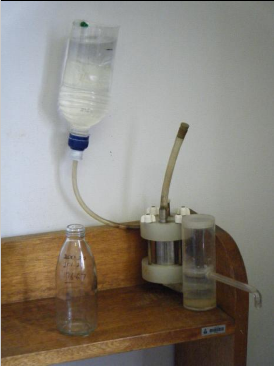
Figure 19: Apparatus used in the Darcy Experiment.
