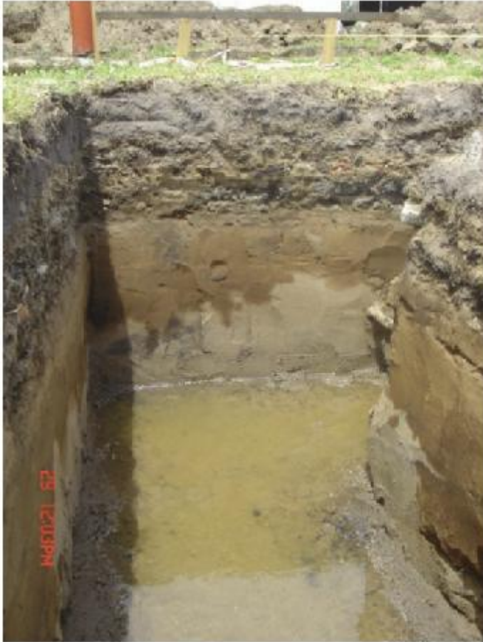
Figure 24: Excavation at the project site showing the unconsolidated layers. Water fingers can be observed on the bottom sand layer.
