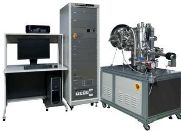
Figure 3.4 PHI 5000 Versa Probe II Scanning XPS Microprobe [7].
