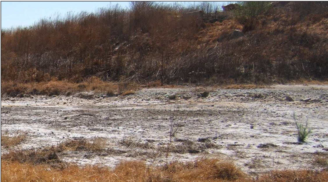
Figure 7: Salt precipitation from the leachate produced by the Charlie I landfill site Sasol Synfuels – Secunda.
