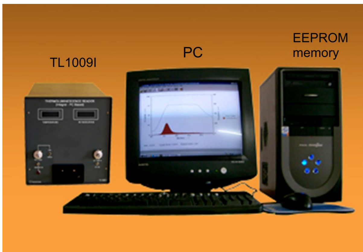
Figure 4.16: Thermoluminescence Reader Type TL1009I designed and offered by Nucleonix Systems Pvt. Ltd., India [35].
