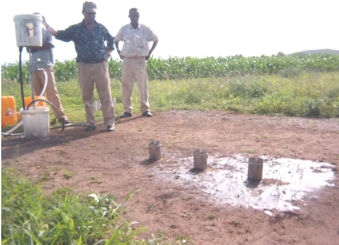
Figure 3. 2 Sprinkler infiltrometer and infiltration rate measurement photograph at Melkassa Hypo Calcic Regosol ecotope.
