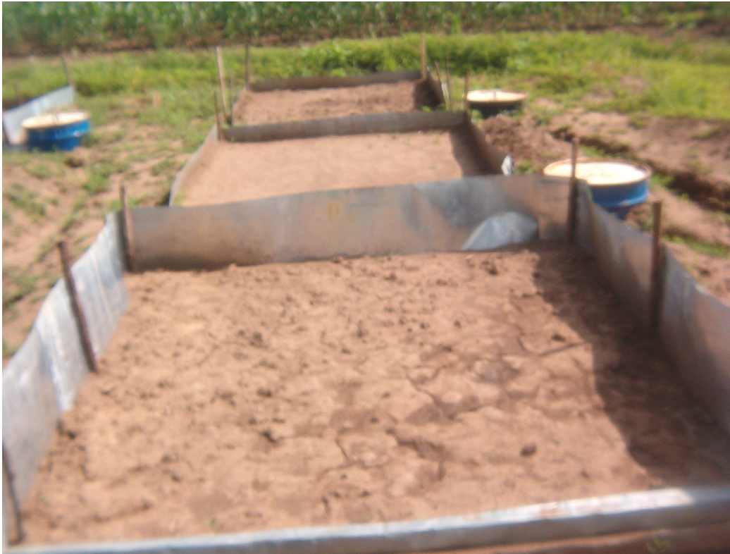
Figure 5. 7 Runoff plots at Melkassa during 2004 showing the development of crust and high SD_m condition on the CT plots (front and rear plots).
