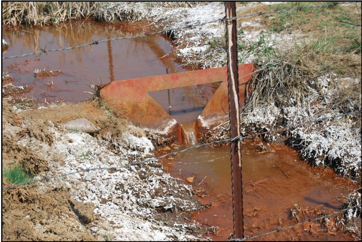
Figure 86: Picture of the V-notch of water decanting out of opencast 1B.
