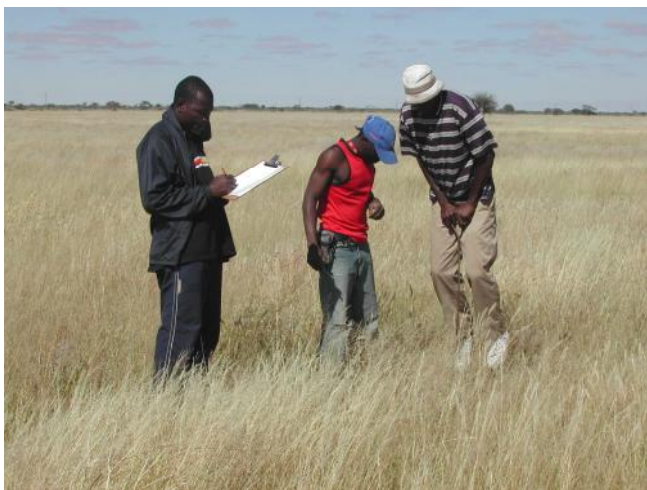
Figure 3.6 Jumping on the top of a soil probe to press it into the ground at Site 22b to determine compaction of the soil by measuring how deep it penetrated.
