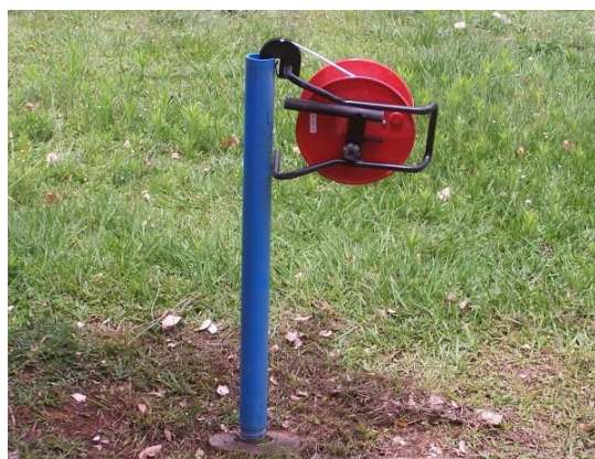
Fig 31: Measuring EC and Water Levels using a TLC meter
