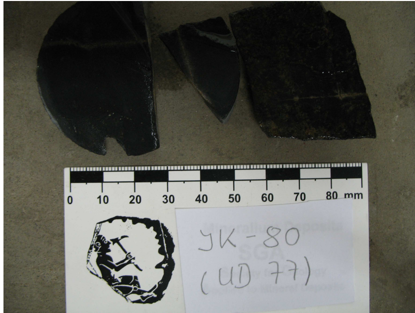
Fig. 5.3: Specimens of Timeball Hill Shale; borehole UD 77
