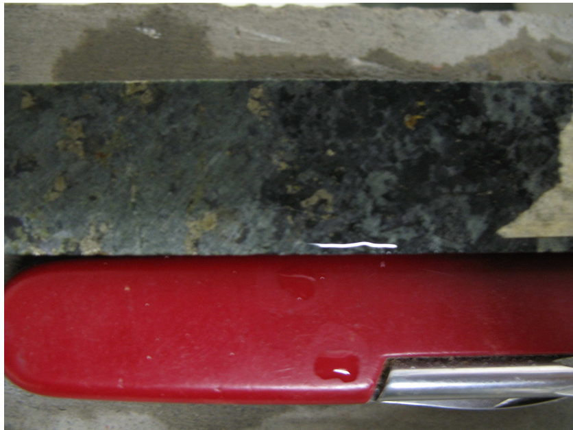
Fig. 5.4: Timeball Hill Shale with mineralization of pyrite
