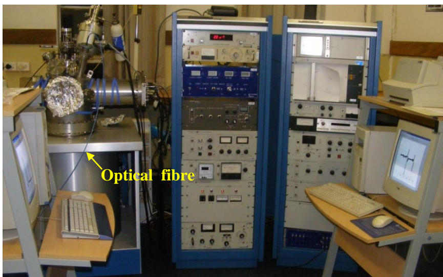
Figure 3.7: The PHI model 549 Auger spectrometer.
