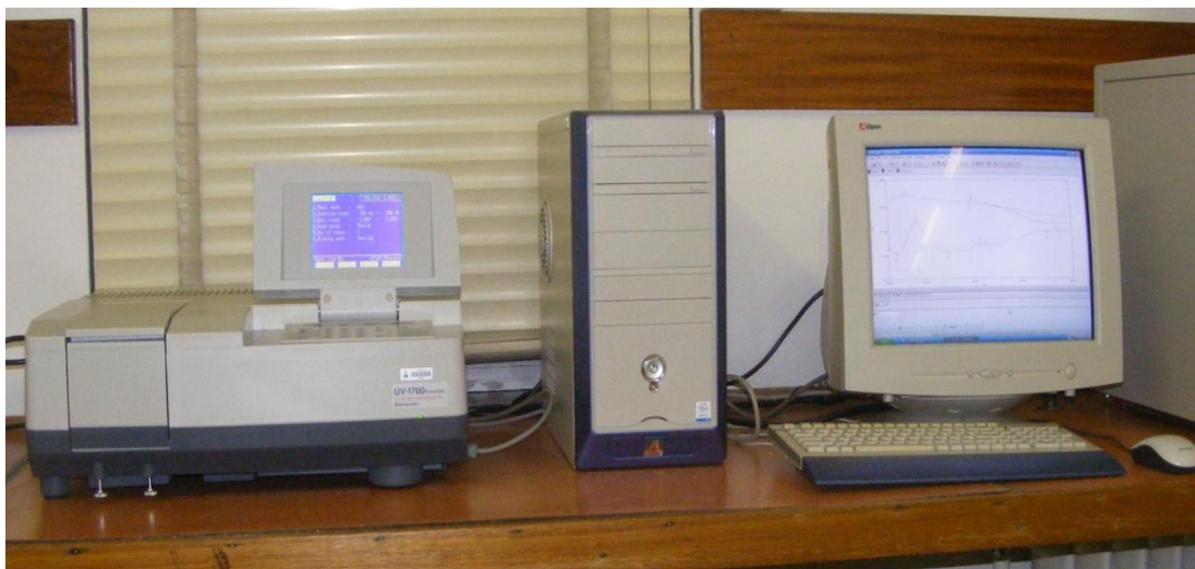
Figure 3.11: UV-1700 PharmaSpec UV-Vis spectrophotometer.
