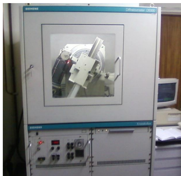
Figure 3.2: Siemens D5000 model x-ray diffractometer
