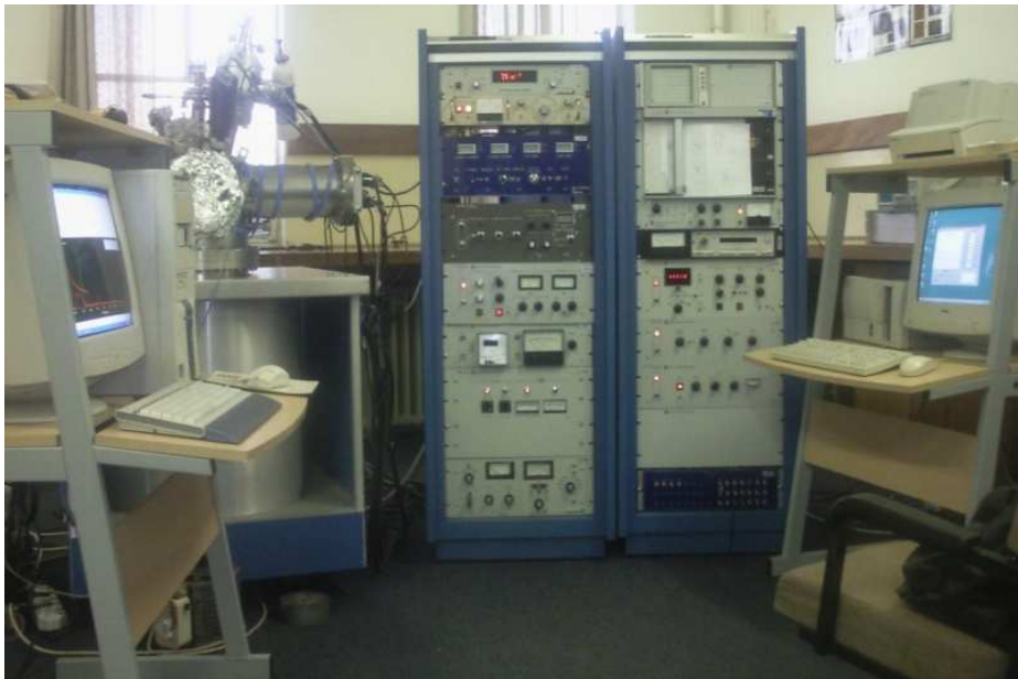
Fig. 2.9 PHI model 549 Auger Electron Spectroscopy (AES) unit coupled with the CL unit at the University of the Free State, Physics department.
