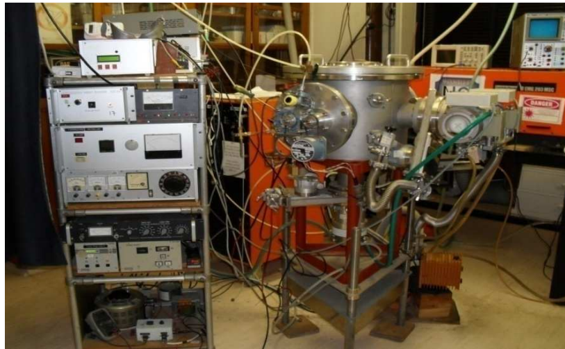
Fig. 2.3 The Pulsed Laser Deposition (PLD) machine at Stellenbosch University, Physics department.
