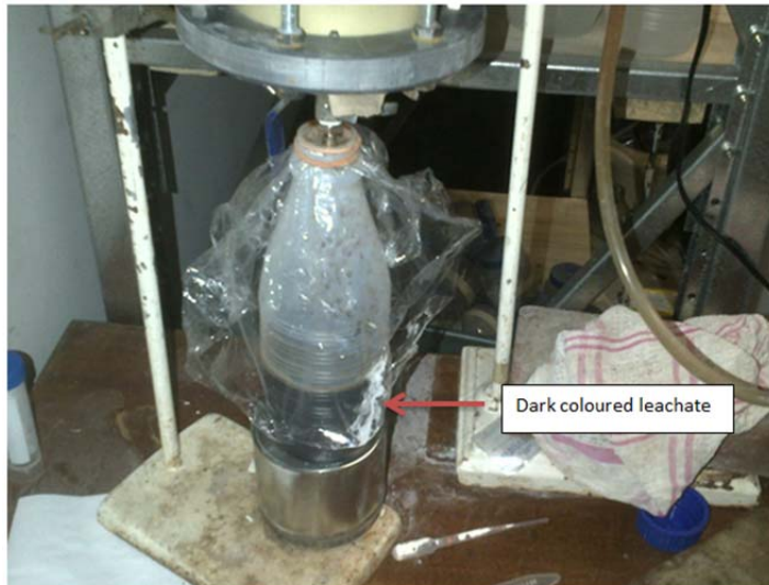
Figure 4-5 Specimen LS2 being leached under a constant head test, dark colour of lignosulphonate dominant in the leachate.
