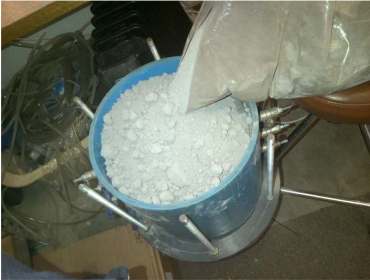
Figure 3-19 Tutuka fly ash being added on top of the multi- layer liner system
