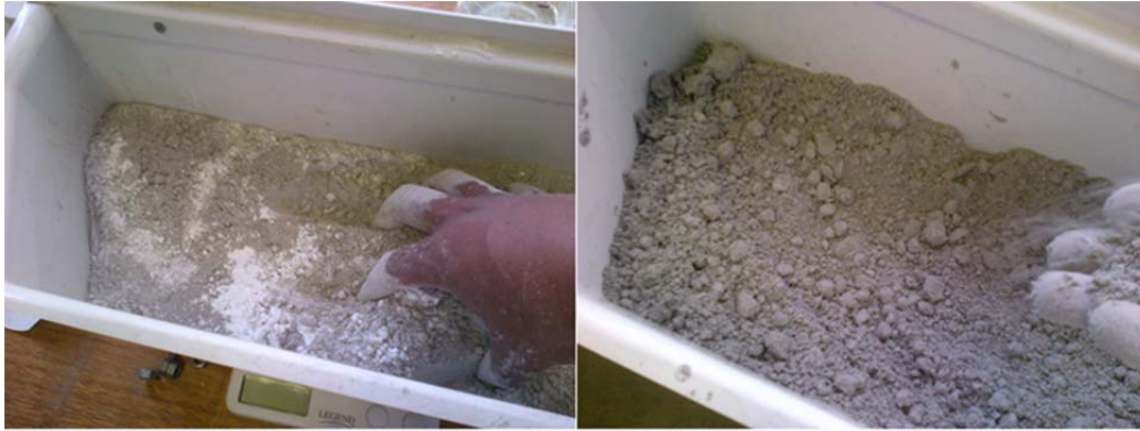
Figure 3-13 Sample mixing, (left) gypsum and lime just added to fly ash, (right) homogeneous mixture of fly ash, gypsum and lime after vigorous mixing
