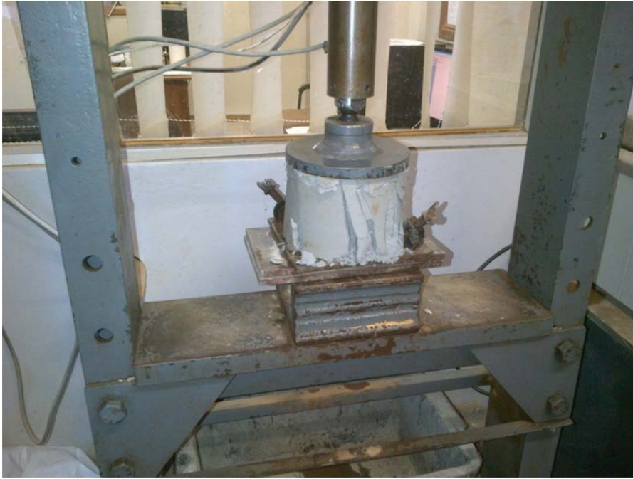
Figure 3-6 Unconfined compression strength test on a fly ash admix sample
