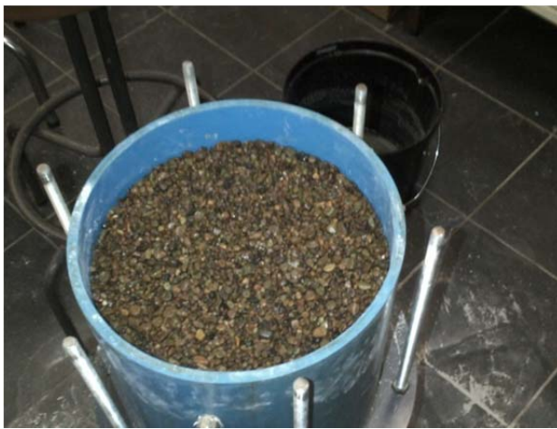
Figure 3-18 Gravel layer inside permeameter cell
