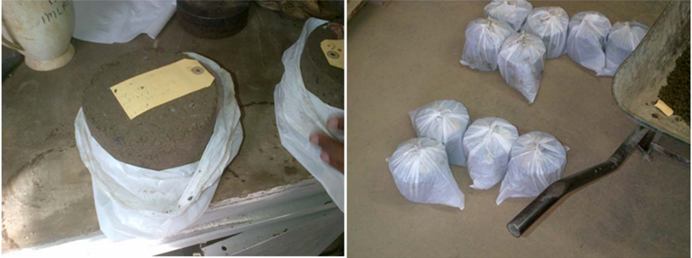
Figure 3-4 Specimens being prepared for rapid curing. The plastic bags create a constant humid environment around the specimens as they were cured for 48 hours in the oven at 60 °C
