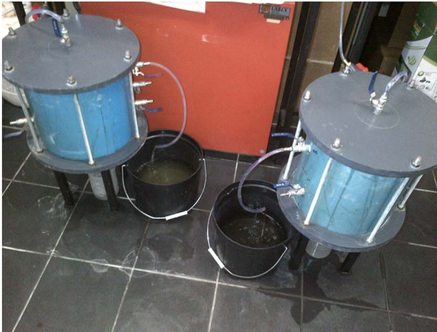
Figure 3-21 Permeameter enclosing multi-layer liner system, left quarter compaction, right full compaction
