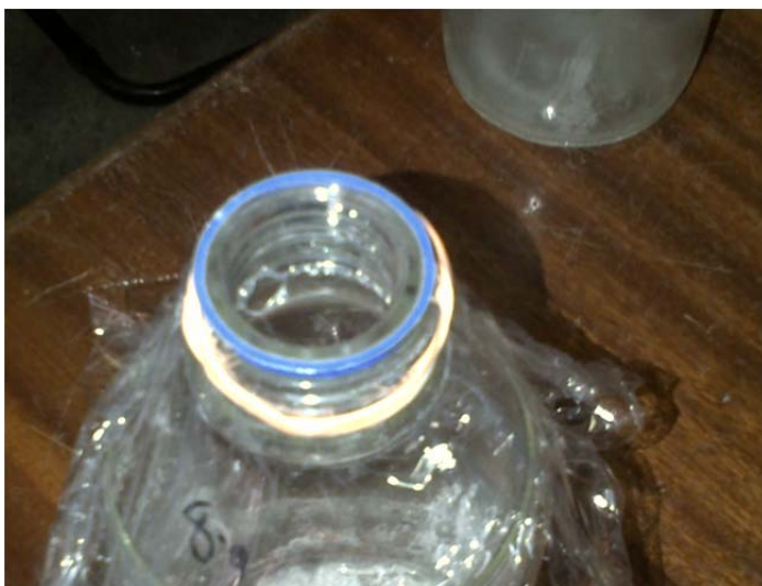
Figure 3-22 Adhesive plastic covering collecting bottle to avoid losses due to gravity
