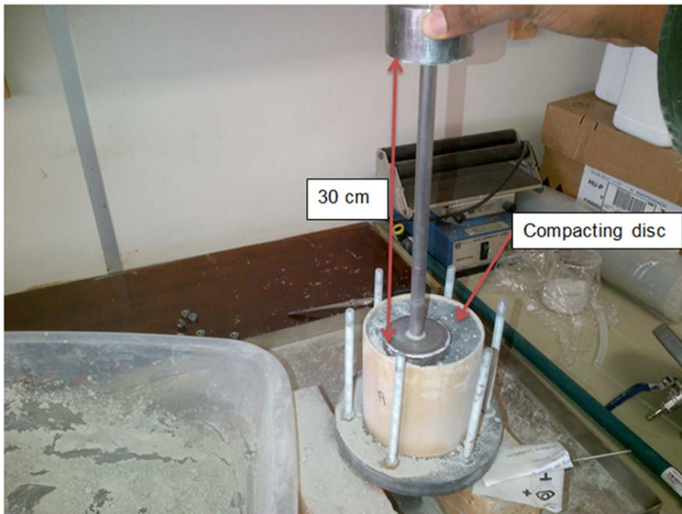
Figure 3-14 Compaction of samples into a column
