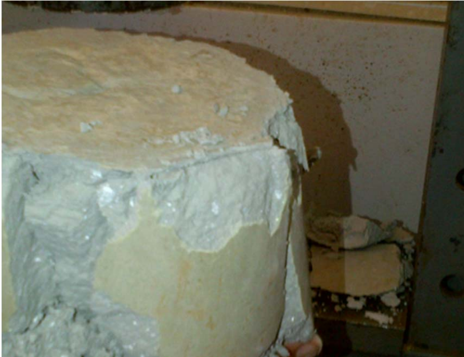
Figure 4-2 White patches of unreacted lime in LSM 9 after ITS crushing
