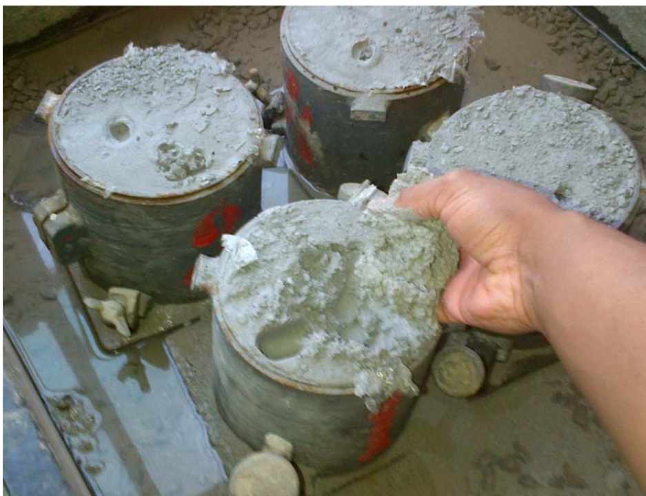
Figure 4-3 Dura-Pozz fly ash collapses in a water bath during curing
