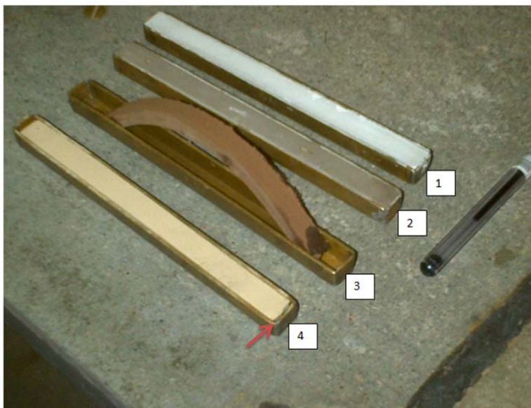
Figure 4-4 Specimens in troughs after oven drying. Specimen 1 in the picture is LSM 7, 2 is LS 2, 3 is clay which has undergone ductile deformation upon drying and 4 is soil-clay mixture that has contracted lineally. This can be seen by the departure from the trough walls (red arrow). 3 and 4 were included for demonstration purposes only.
