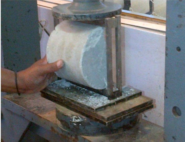
Figure 3-7 Sample splits in half during an indirect tensile strength test
