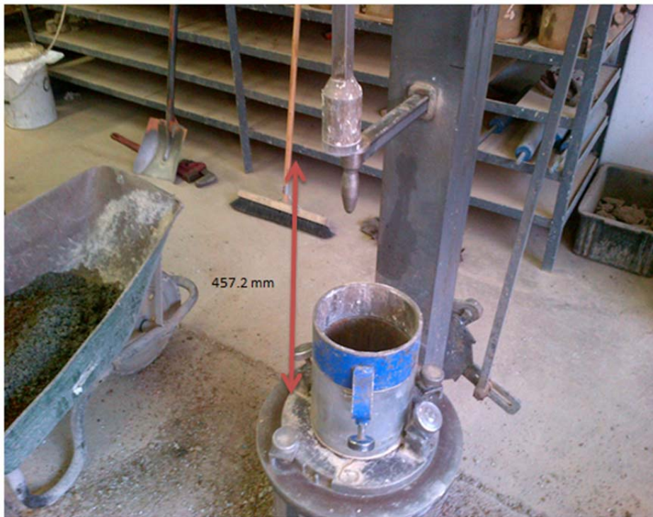
Figure 3-2 Mould under a tamper during compaction
