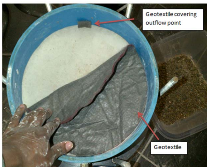
Figure 3-17 Geotextile being placed on top of compacted layer, also a small piece of geotextile is placed at an outflow point to prevent clogging of the pipe
