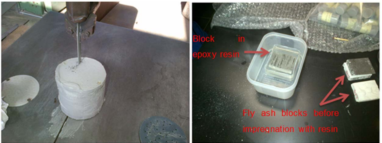
Figure 3-11 Preparation of block samples, left sample from permeameter is being cut, right is square blocks of samples
