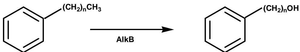
Figure 2.12: Hydroxylation of alkylbenzenes by the alkane hydroxylase system of P. oleovorans Gpo1. n=1 is ethylbenzene, and the product of hydroxylation is 2-phenyl-1-ethanol; n=2 is propylbenzene and the product is 3-phenyl-1-propanol; n=3 is butylbenzene and the product is 4-phenyl-1-butanol (van Beilen et al. , 1994).
