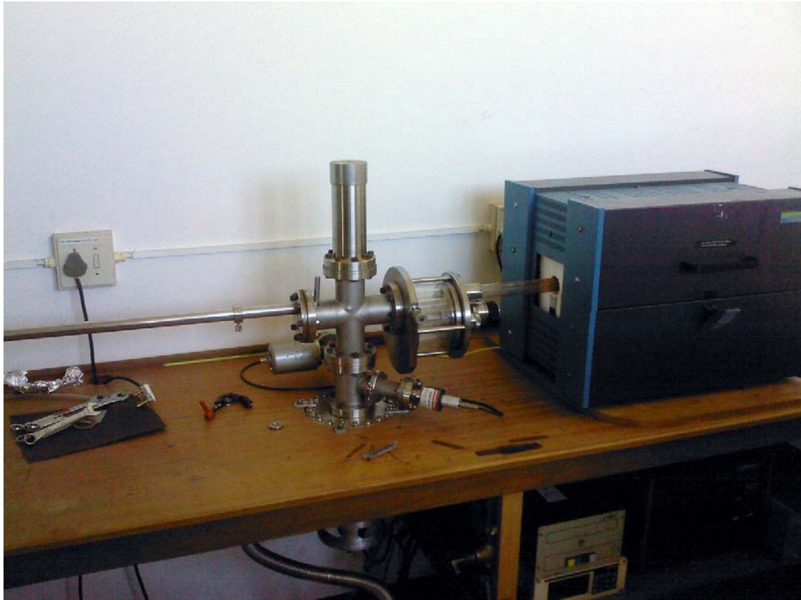
Figure 5.2: Picture of the custom built vacuum annealing system used during the course of this study.
