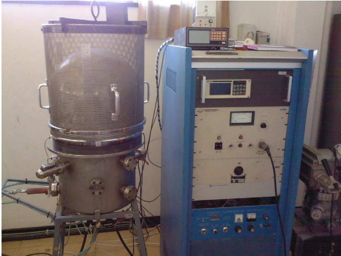
Figure 5.1: Picture of the electron beam physical vapour deposition system used during the course of this study.
