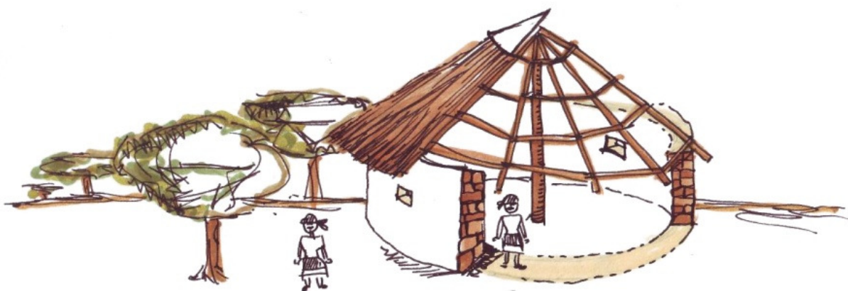
Figure 3.2: Cross section of a traditional isiXhosa hut displaying various material properties that ensure thermal stability
