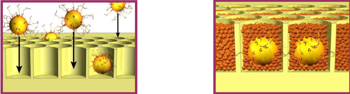
Figure 4.1. Optimized bead deposition within the picotitre plate. The size of the wells along with the size of the beads are optimized in such a way that only one library bead fits into one well along with enzyme beads for the sequencing reaction and packing beads for holding each bead within a well (Mardis, 2008).
