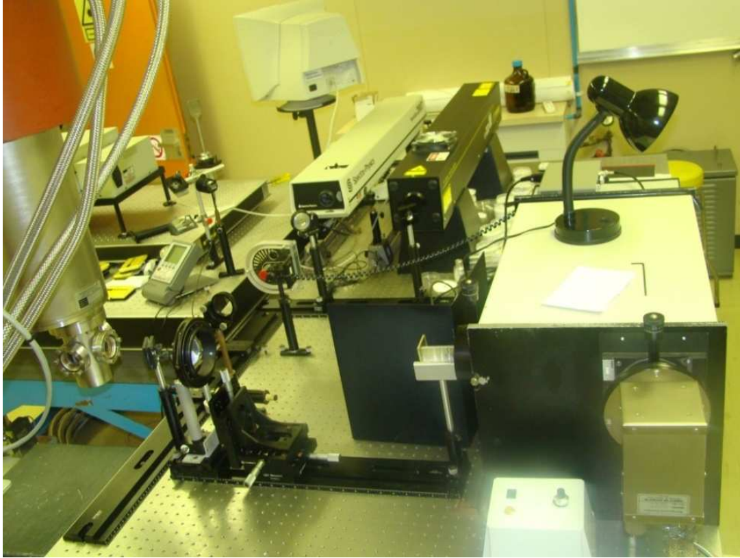
Figure 3.7: PL system used to investigate the luminescent properties of the phosphors.
