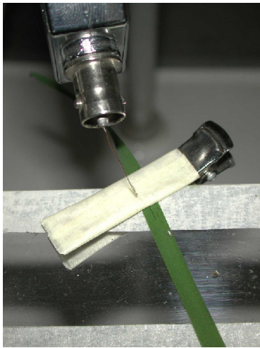
FIGURE 3.3 Close-up of leaf held in position by hairclip and EPG probe with D. noxia wired in position.
