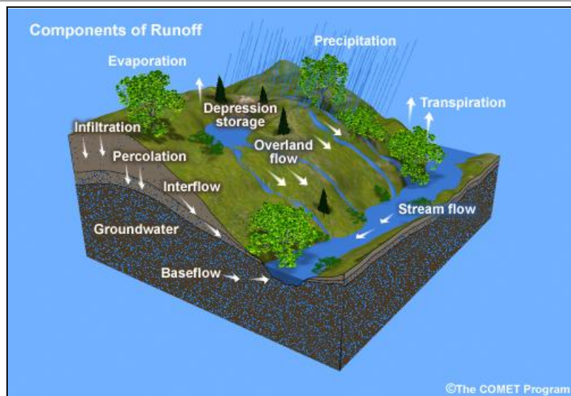
Figure 2-1 The various water sources to a river system. Water can reach the river by means of overland flow, interflow and groundwater discharge (Taken from Schreiber-Abshire, et al. , 2005).
