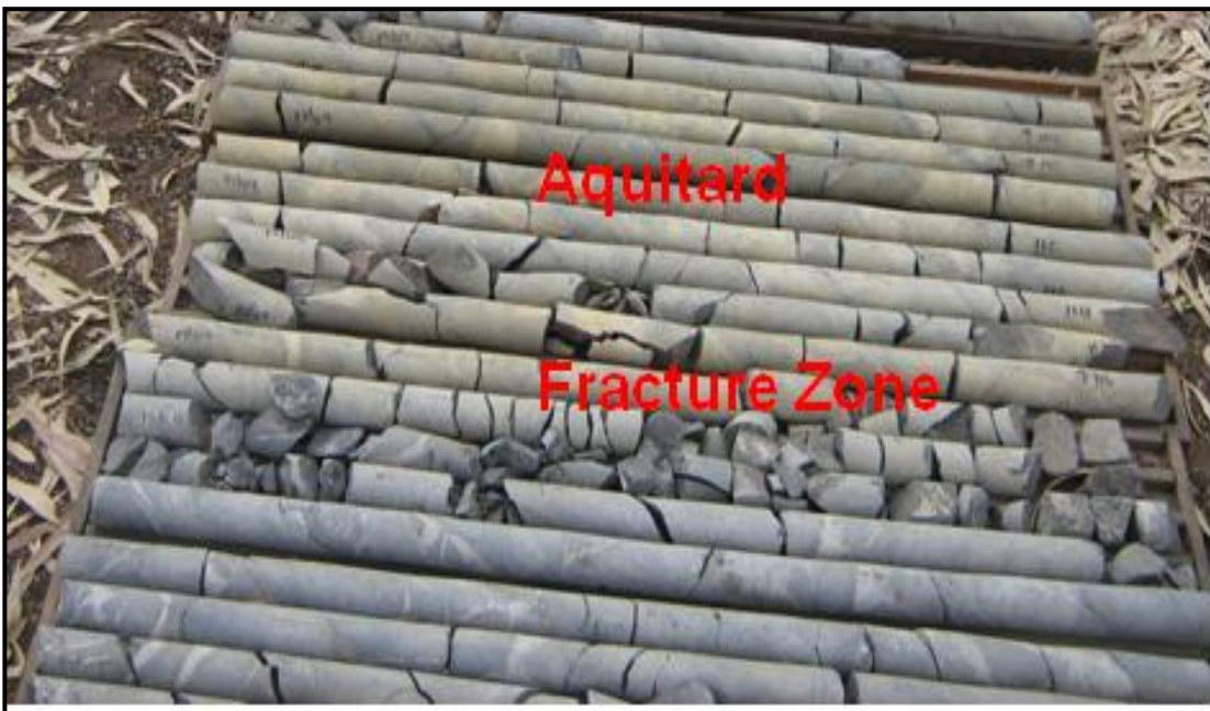
Figure 33: Fracture zone intersected by diamond drilling in the Huttenberg Formation
