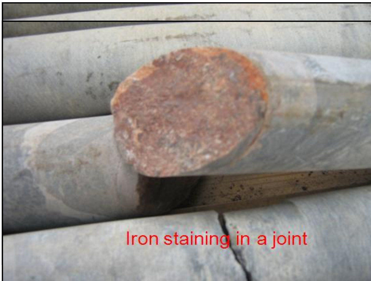
Figure 32: Iron staining in deep-seated joints
