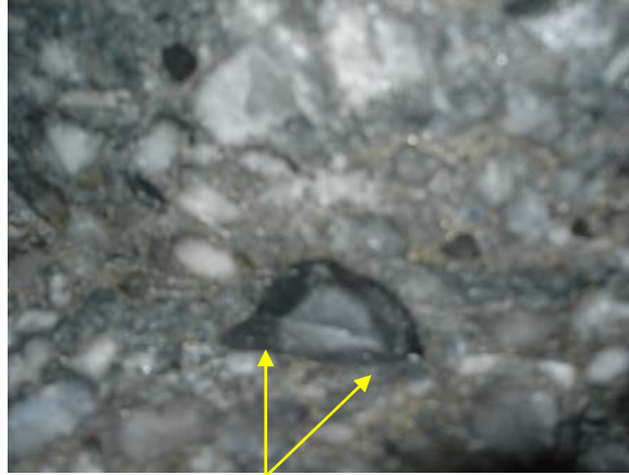
Figure 4.1. Photograph showing the in situ secondary alteration of milky quartz 2 cm in diameter to smoky quartz. Note how the alteration started at the edge of the milky quartz.
