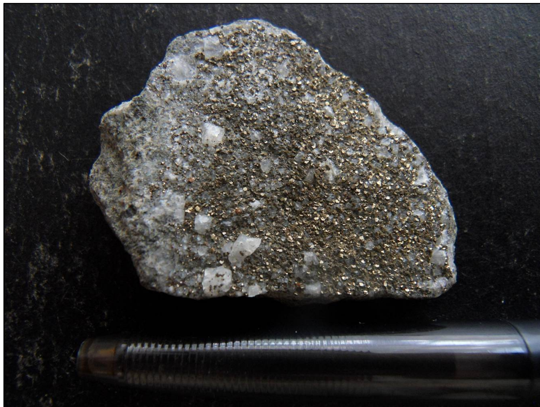
Figure 6-8: Chip (42mm dia.) from EC-Q14-1636 water strike at 122 mbgl with pyrite
