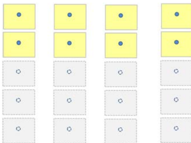
Figure 6-4 Systems approach to sustainable groundwater development and management at Middelburg (40 L/s at 5 L/s/borehole = 8 boreholes).
