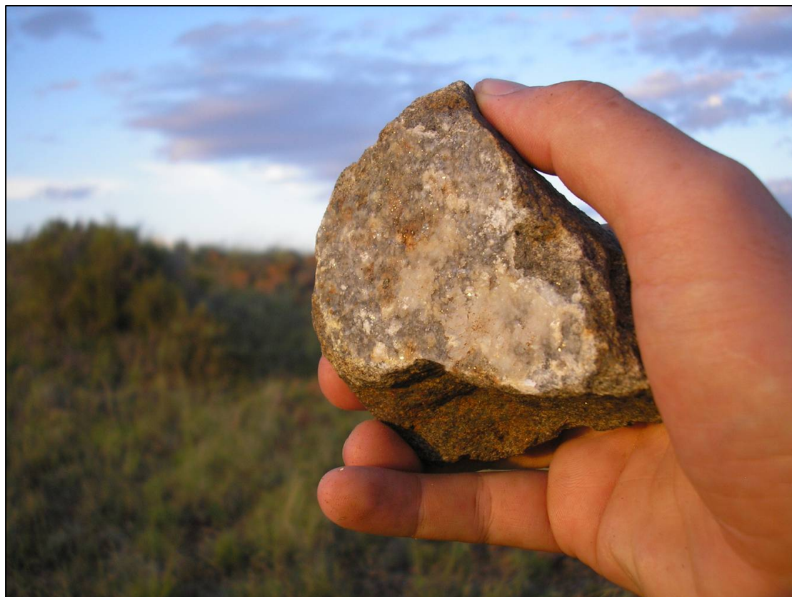
Figure 6-7: Rock expelled from fracture found in EC-Q14-1636 at 122 mbgl
