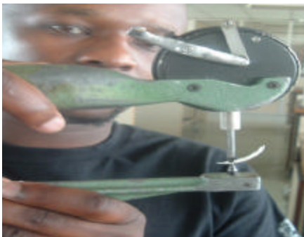
Figure 3.5 Measurement of shell thickness
