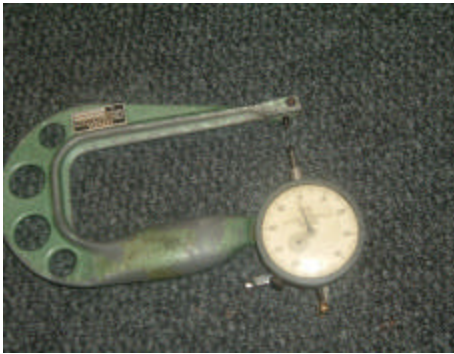
Figure 3.3 Egg thickness meter
