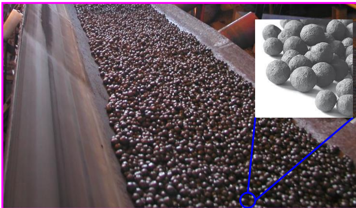
Figure 2-4: Green (wet) pellets on ferrochrome plant conveyor belt (Vehviläinen, 2005)
