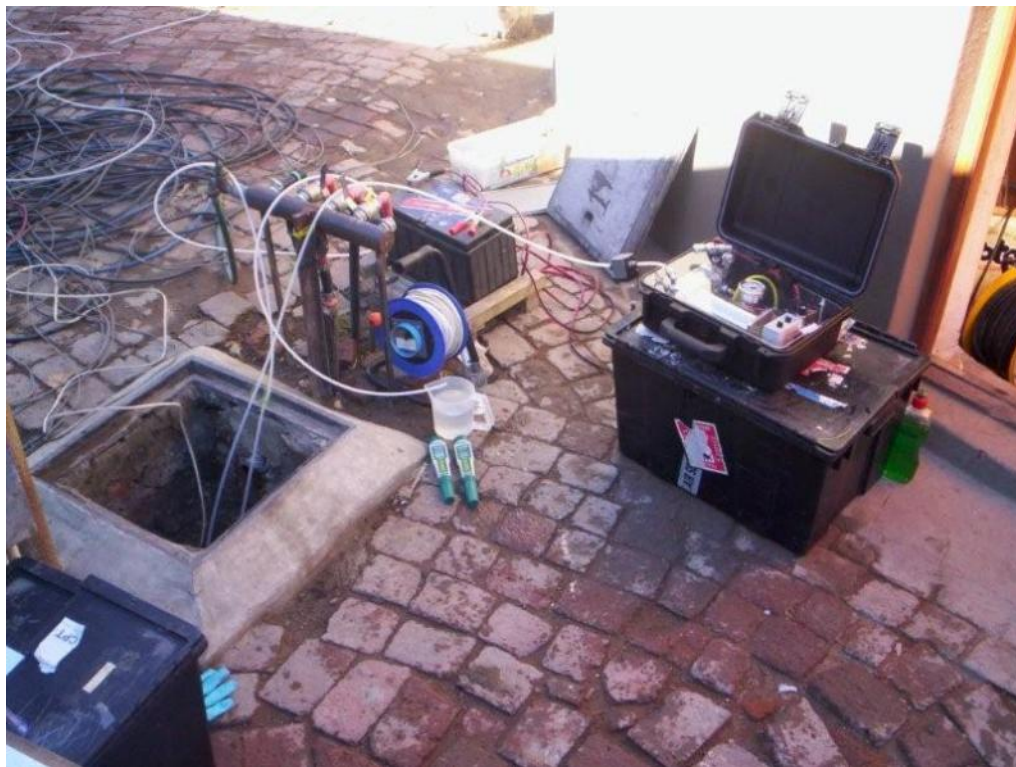
Photo 9-1 Low flow bladder pump sampling of PW9
