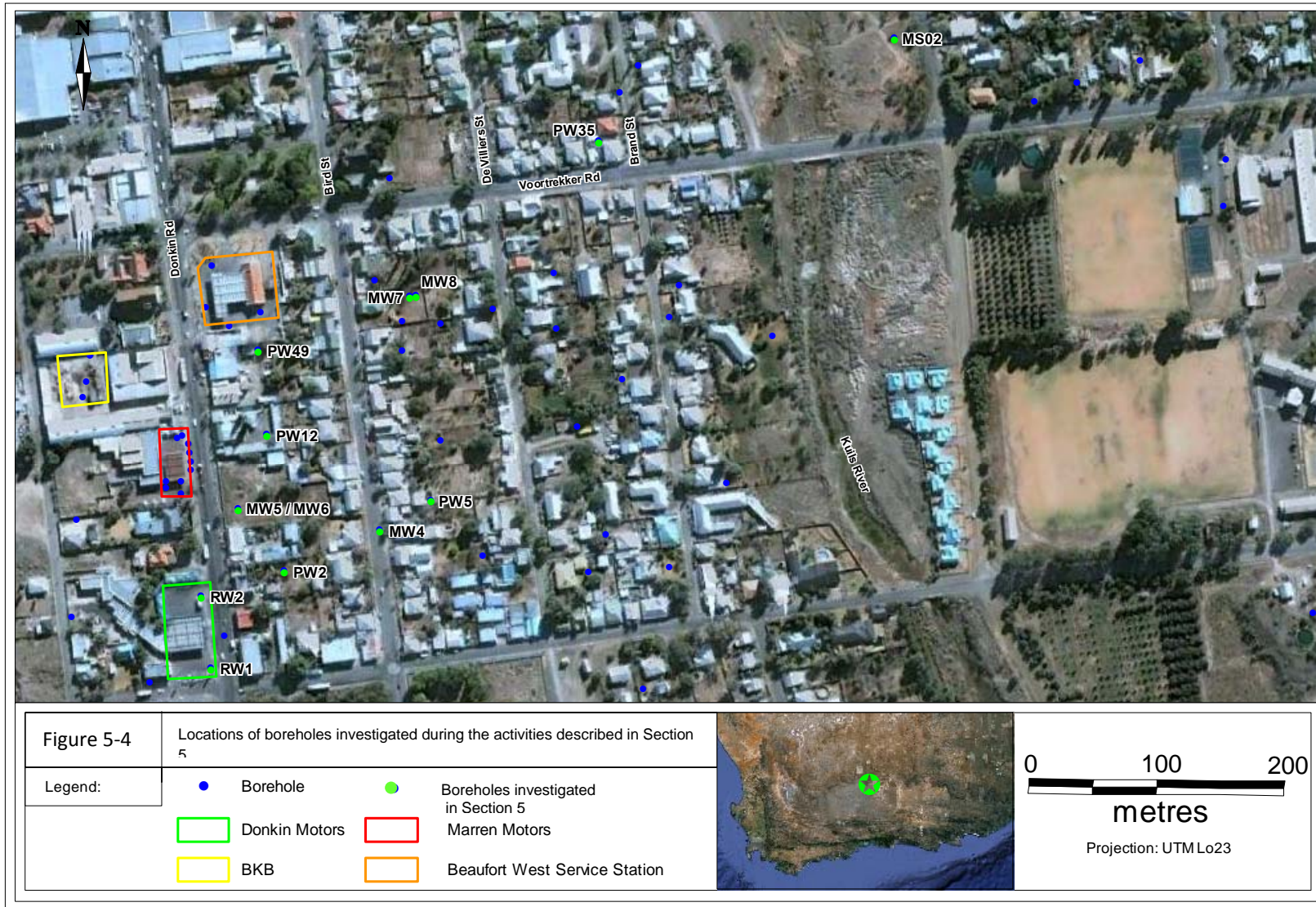
Figure 5-4 Locations of boreholes/monitoring wells investigated during the activities described in Section 5.
