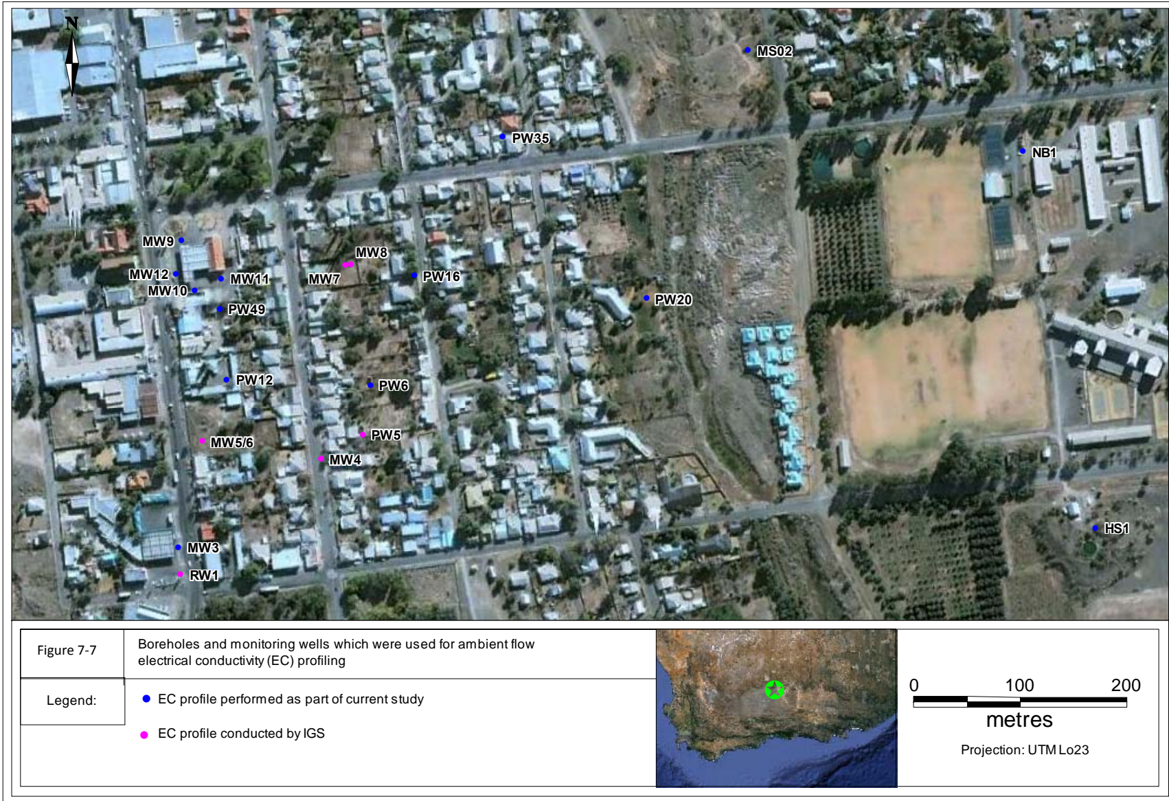
Figure 7-7 Boreholes and monitoring wells which were used for ambient flow electrical conductivity (EC) profiling
