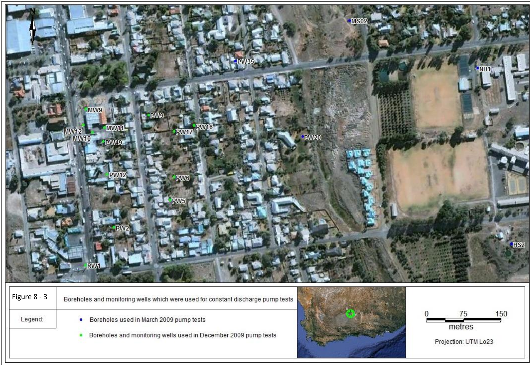
Figure 8-3: Site layout of boreholes and monitoring wells used in constant rate discharge test.
