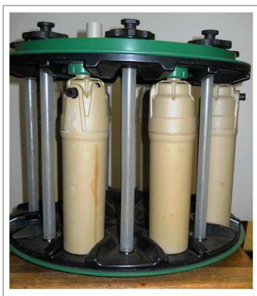
Figure 2-10: Carousel with mounting slots for eight reaction vessels.
