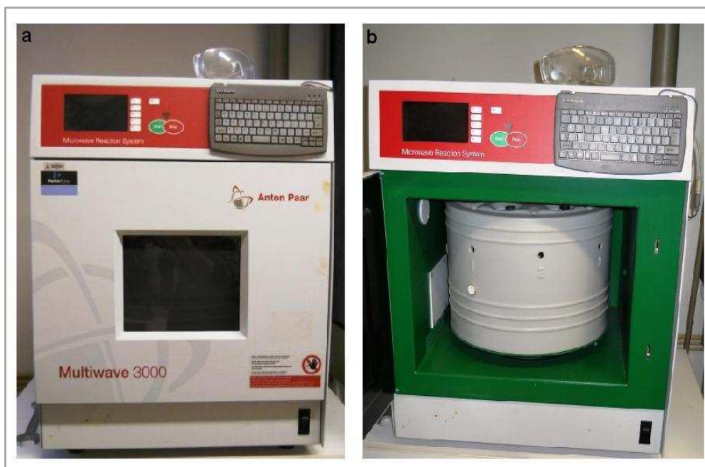
Figure 2-8: (a) Front view of microwave reactor, (b) open view of microwave reactor with carousel visible.
