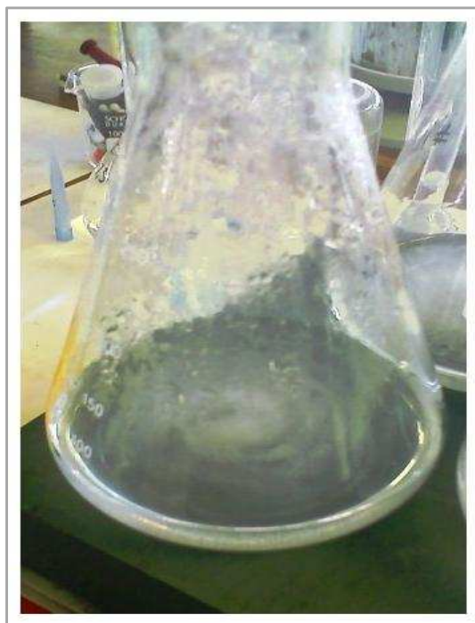
Figure 3-2: Ta metal powder reacting with concentrated KOH solution.
