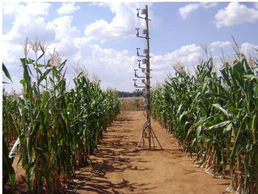
Figure 9.1 Sensor arrangements in the wide runoff section within and above the maize canopy from 1.8m up to the reference height of 4.5 m on 07 April, 2009.
