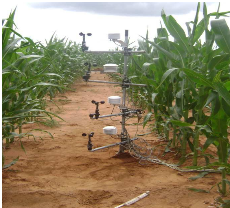
Figure 8.1 Sensor arrangements in the runoff section within the maize canopy at 1.6 m crop height on 25 Feb., 2009 for the 3 m length runoff strip.
